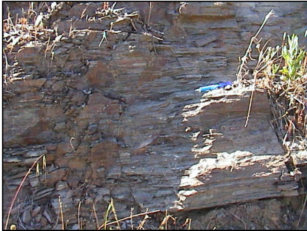
Figure 3.9 A close view of schists from the entrance portal of the Dim Tunnel at Km 6+050.
