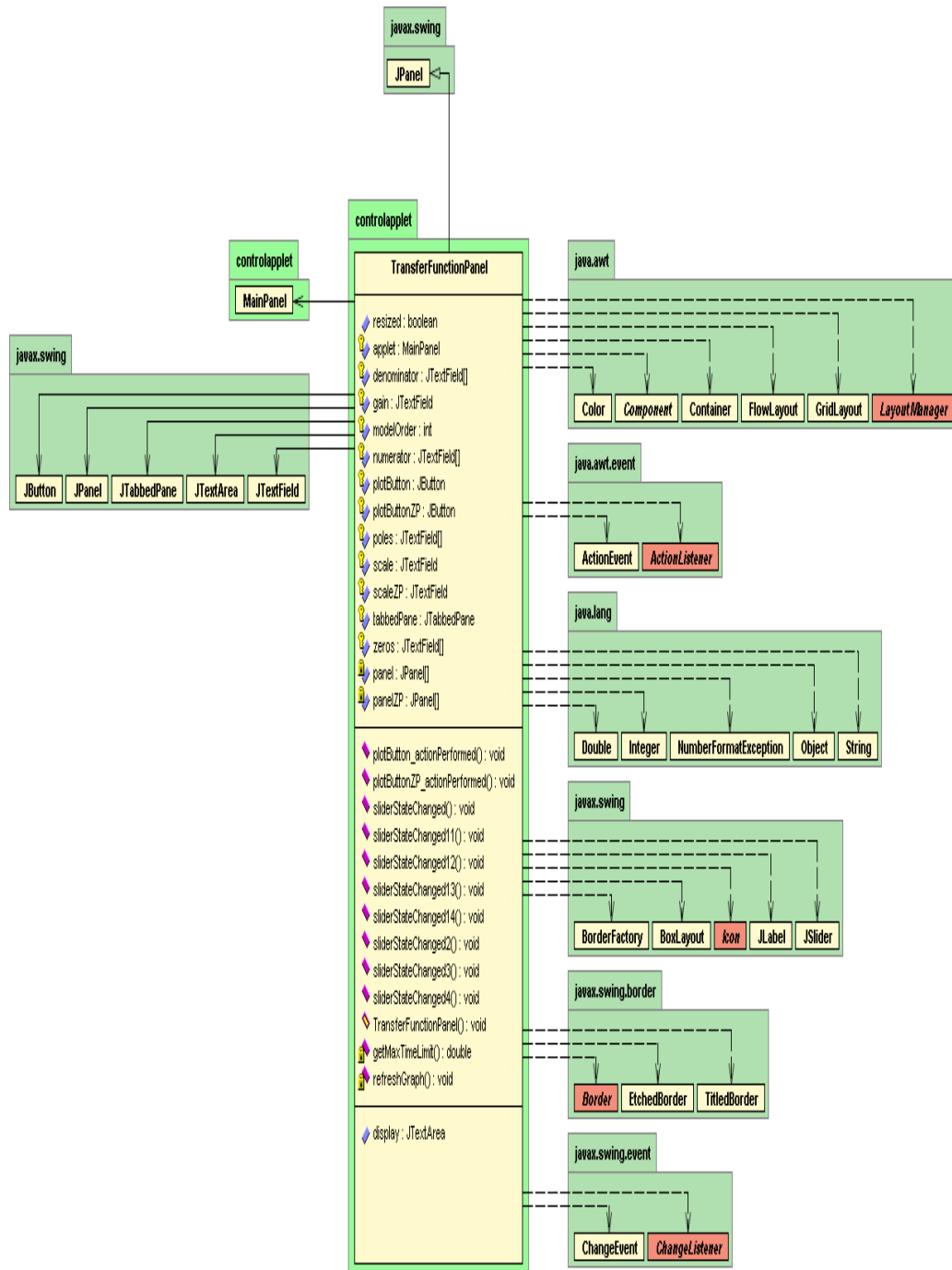
Figure 23 TransferFunctionPanel class in UML notation
