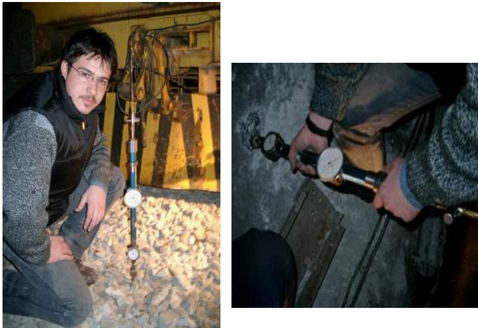
Figure 6.5 Convergence Measurement at a Station
