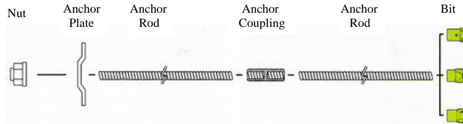
Figure 5.9 Components of MAI Bolt SDA (after Atlas Copco, 2003)
