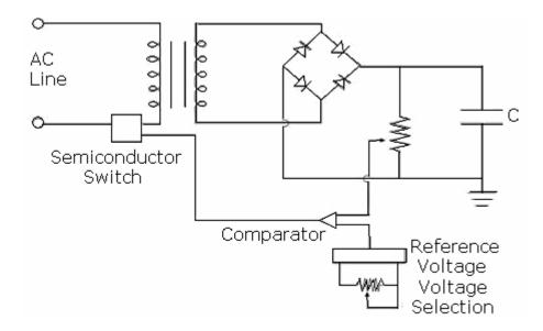
Figure-3.21: Charging supply with SCR control.
