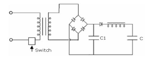
Figure-3.24: Charging supply with resonant charging unit.
