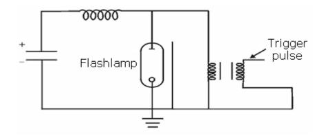
Figure-3.28: Parallel trigger circuit
