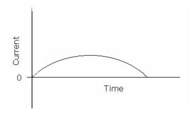
Figure-0.31: Overdamped current waveform from a flashlamp discharge circuit.
