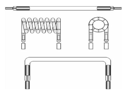
Figure-2.6: Flash lamps with various geometries.
