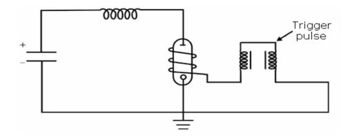
Figure-3.26: External trigger circuit
