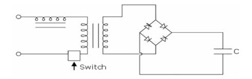
Figure-3.23: Charging supply with current limiting inductor.
