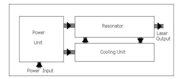
Figure-3.10: Block diagram showing a typical laser
