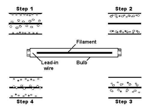
Figure-2.9: Tungsten halogen lamp and halogen cycle.
