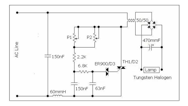
Figure-3.34: Tungsten halogen lamp power supply.
