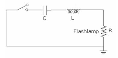
Figure-3.29: RLC discharge circuit
