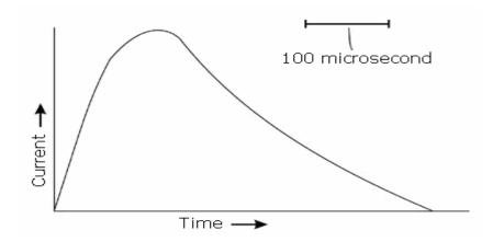
Figure-2.8: Typical waveform for a flashlamp current pulse lasting a few hundred microseconds.
