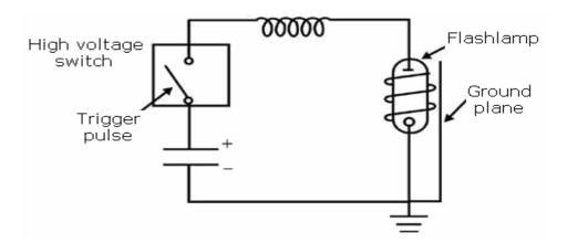
Figure-3.25: Overvoltage trigger circuit.
