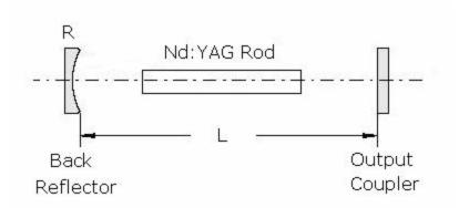
Figure-3.11: Hemispherical resonator. R= 2.0 m.
