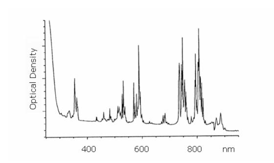
Figure-2.5: Spectral absorption of Nd:YAG
