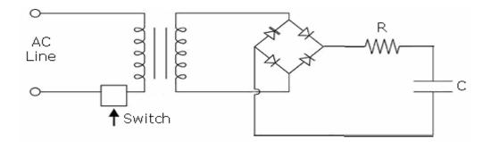
Figure-3.22: Charging supply with current limiting resistor.
