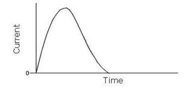
Figure-3.32: Critically damped current waveform from a flashlamp discharge circuit.
