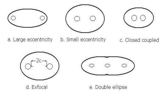
Figure-3.12: Elliptical pump cavities.
