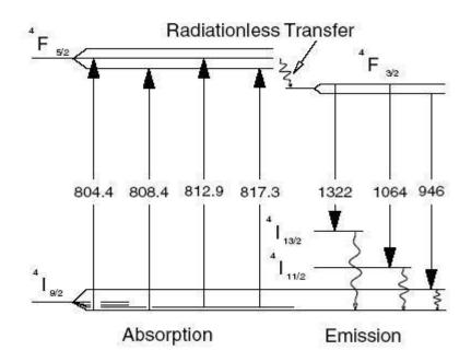
Figure-2.1.: Absorption and emission levels of Nd:YAG
