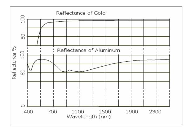
Figure-3.16: Spectral reflectance of gold and aluminum.
