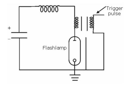
Figure-3.27: Series trigger circuit
