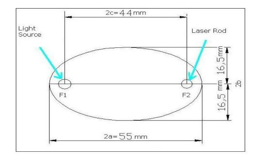
Figure-3.14: Cross section of elliptical cavity with small eccentricity. The cover is aluminum with dimensions: 91x102x85 in mm.
