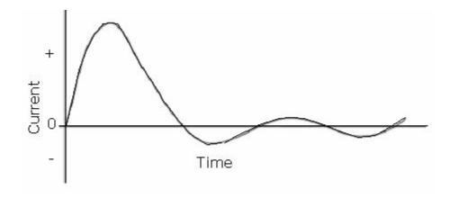
Figure-3.30: Underdamped current waveform from a flashlamp discharge circuit.
