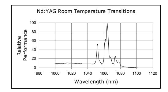
Figure-4.2: Measured Nd:YAG room temperature transitions above 1000nm.
