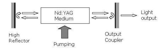
Figure-2.4: Gain process, resonator and Nd:YAG medium
