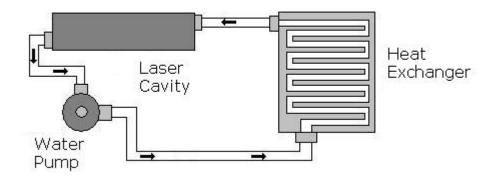
Figure-3.35: Closed loop cooling system.
