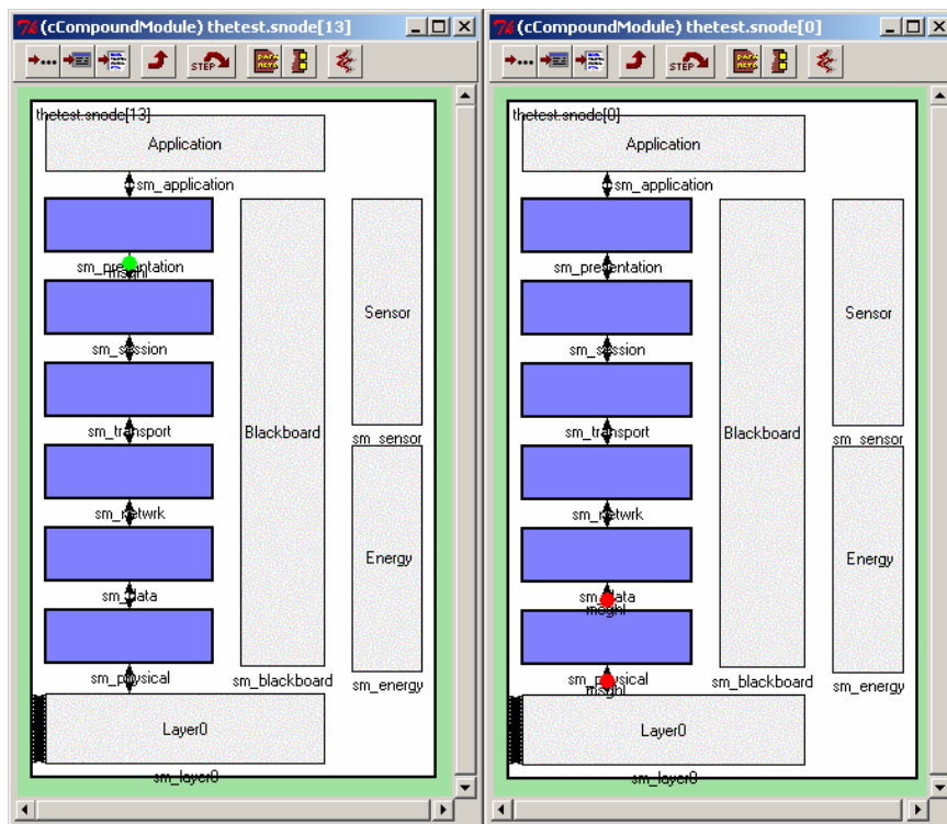
Figure 5. Two snapshots of the sensor nodes, first one just generated the message but second one is about to send it
