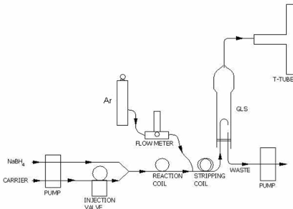
Figure 2.3 Schematic Diagram of the FI-VGAAS System.
