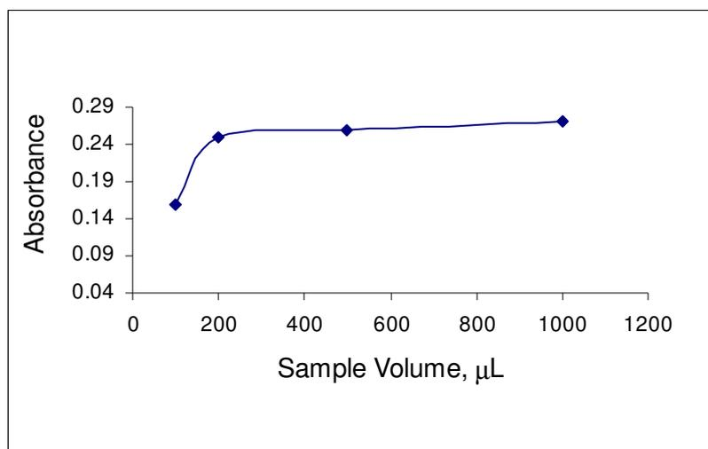
Figure 3.10 Variation of Ag Signal, with sample volumes for  $1.0 \text{ mg L}^{-1}$  Ag in  $3.0 \text{ M HNO}_3$ ; using carrier acid  $3.0 \text{ M HNO}_3$ ,  $0.5\%$  (w/v)  $\text{NaBH}_4$  in  $0,1\%$  (w/v)  $\text{NaOH}$ , argon flow  $85 \text{ mL min}^{-1}$ , reaction coil  $4.0 \text{ cm}$ , stripping coil  $25.0 \text{ cm}$ .
