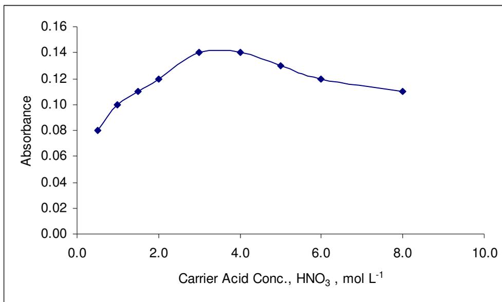
Figure 3.5 Effect of Carrier Acid, HNO<sub>3</sub>, using 0.1 mL of 1.0 mg L<sup>-1</sup> Ag in 3.0 M HNO<sub>3</sub>, 0.5% (w/v) NaBH<sub>4</sub> in 0,1% (w/v) NaOH, argon flow 85 mL min<sup>-1</sup>, reaction coil 4.0 cm, stripping coil 25.0 cm.
