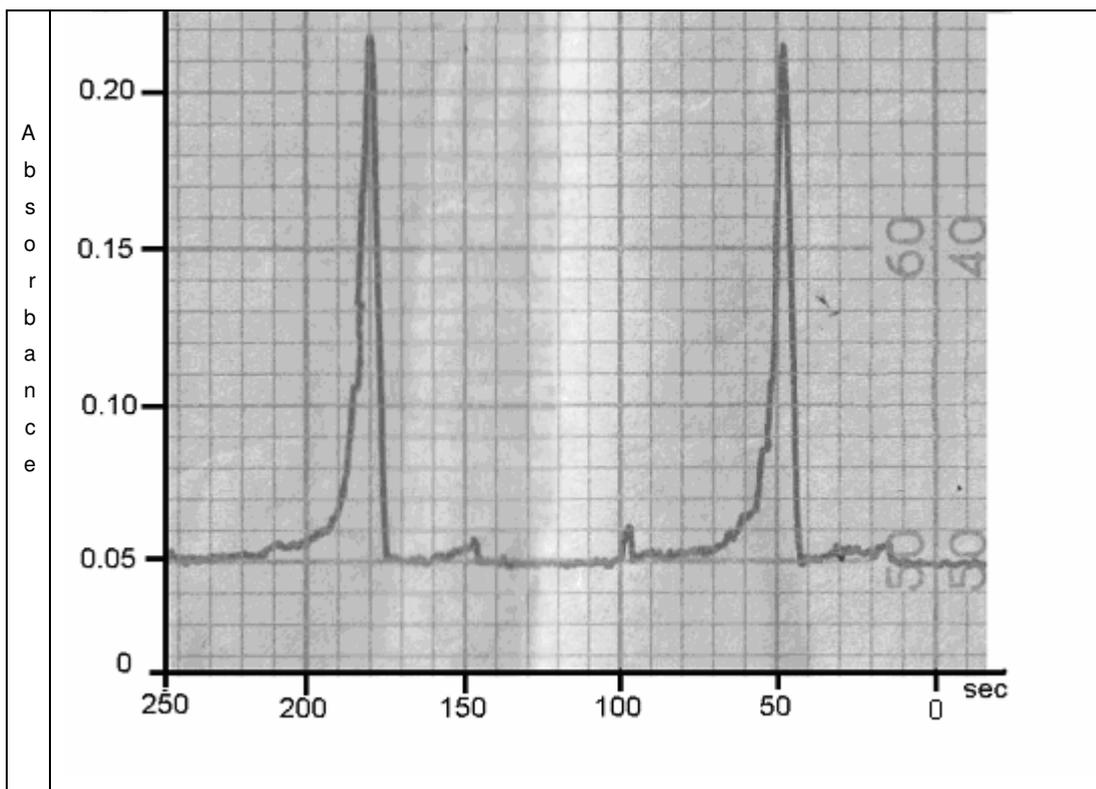
Figure 3.4 Transient Signal of Ag using 1.0 M HNO<sub>3</sub> as a carrier acid with U-shaped GLS, for 0.1 mL of 1.0 mg L<sup>-1</sup> Ag in 0.6 M HNO<sub>3</sub>, 0.8% (w/v) NaBH<sub>4</sub> in 0,1% (w/v) NaOH, argon flow 357 mL min<sup>-1</sup>.
