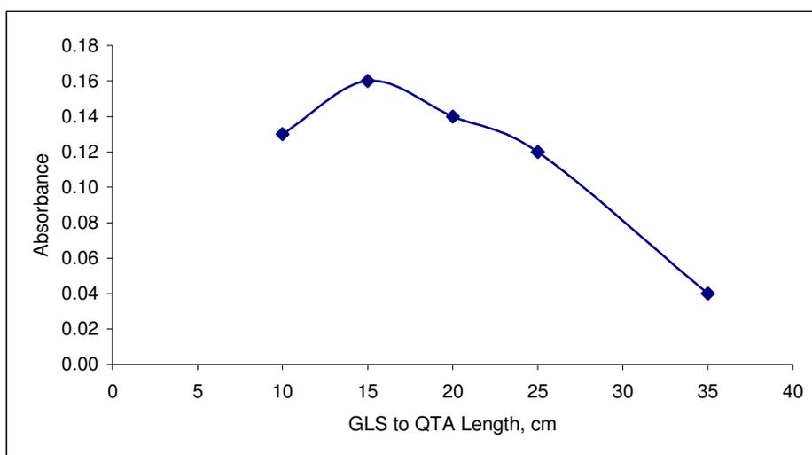
Figure 3.9 Effect of Tubing Length between GLS and QTA on Ag Signal; using 0.1 mL of 1.0 mg L<sup>-1</sup> Ag in 3.0 M HNO<sub>3</sub>, carrier acid 3.0 M HNO<sub>3</sub>, 0.5% (w/v) NaBH<sub>4</sub> in 0,1% (w/v) NaOH, argon flow 85 mL min<sup>-1</sup>, reaction coil 4.0 cm, stripping coil 25.0 cm.
