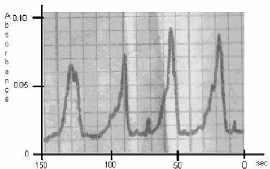
Figure 3.11 Transient Signals of Freshly Cleaned CVG –AAS System; using 0,1 mL of  $1.0 \text{ mg L}^{-1}$  Ag in 3.0 M  $\text{HNO}_3$ , carrier acid 3.0 M  $\text{HNO}_3$ , 0.5% (w/v)  $\text{NaBH}_4$  in 0,1% (w/v)  $\text{NaOH}$ , argon flow  $85 \text{ mL min}^{-1}$ , reaction coil 4.0 cm, stripping coil 25.0 cm.
