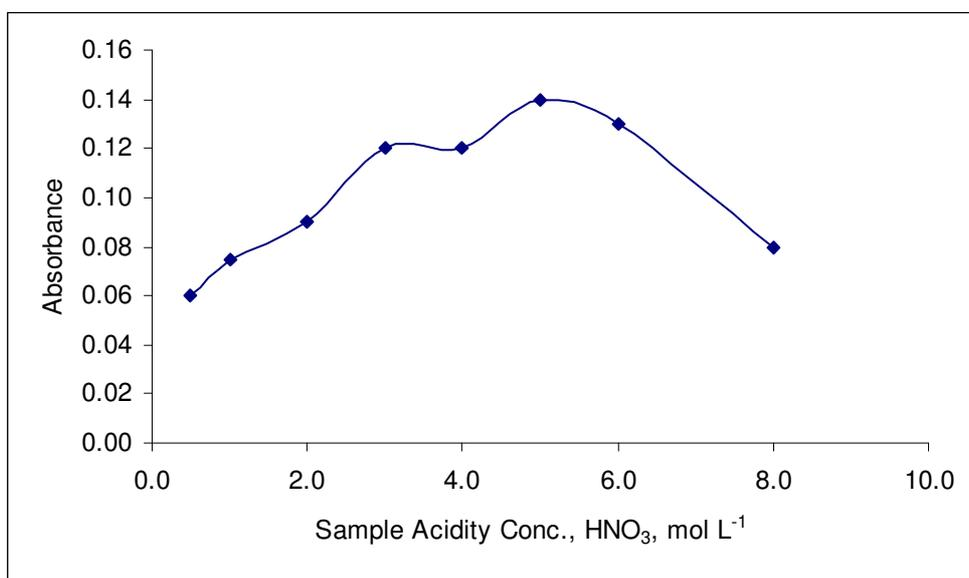
Figure 3.6 Effect of Sample Solution Acidity, HNO<sub>3</sub>, using carrier acid 3.0 M HNO<sub>3</sub>, 0.5% (w/v) NaBH<sub>4</sub> in 0,1% (w/v) NaOH, argon flow 85 mL min<sup>-1</sup>, reaction coil 4.0 cm, stripping coil 25.0 cm.
