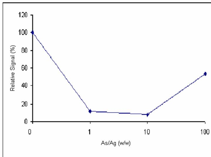
Figure 3.19 Interference of Arsenic on Ag CVG Signal
