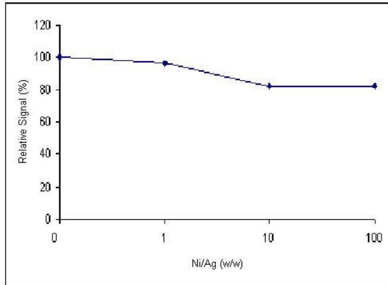
Figure 3.14 Interference of Nickel on Ag CVG Signal
