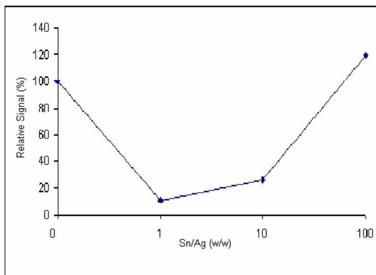
Figure 3.22 Interference of Tin on Ag CVG Signal
