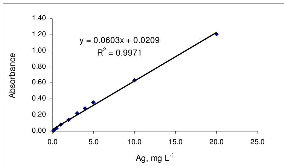
Figure 3.24 Calibration Graph for Ag Determination by FAAS.
