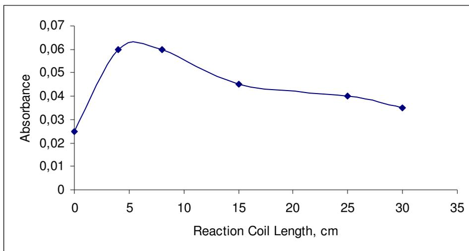
Figure 3.7 Effect of Reaction Coil Length, using 0.1 mL of 1.0 mg L<sup>-1</sup> Ag in 1.5 M HNO<sub>3</sub>, carrier acid 1.5M HNO<sub>3</sub>, 1.0% (w/v) NaBH<sub>4</sub> in 0,1% (w/v) NaOH, argon flow 76 ml min<sup>-1</sup>, stripping coil 35.0 cm.
