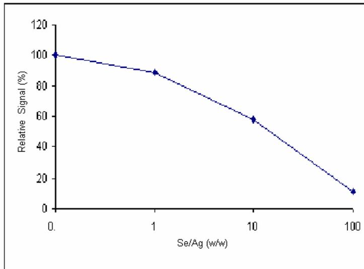
Figure 3.21 Interference of Selenium on Ag CVG Signal
