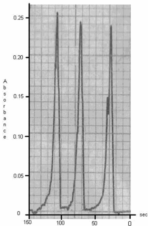
Figure 3.13 Transient Signal of CVG –AAS System Coated with 6.0 mL of  $20.0 \text{ mg L}^{-1}$  Pd and then 7.0 mL of  $1.0 \text{ mg L}^{-1}$  Ag were passed through the system; using 0.1 mL of  $1 \text{ mg L}^{-1}$  Ag in 3.0 M  $\text{HNO}_3$ , carrier acid 3.0 M  $\text{HNO}_3$ , 0.5% (w/v)  $\text{NaBH}_4$  in 0,1% (w/v)  $\text{NaOH}$ , argon flow  $85 \text{ mL min}^{-1}$ , volume 0.1 mL, reaction coil 4.0 cm, stripping coil 25.0 cm.
