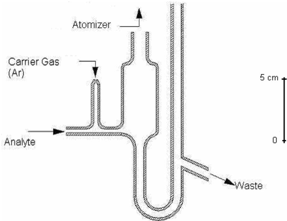
Figure 2.1 U-shaped Gas-Liquid Separator Design
