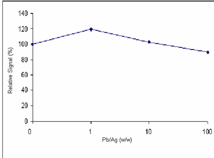
Figure 3.20 Interference of Lead on Ag CVG Signal
