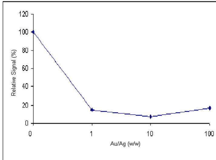
Figure 3.18 Interference of Gold on Ag CVG Signal
