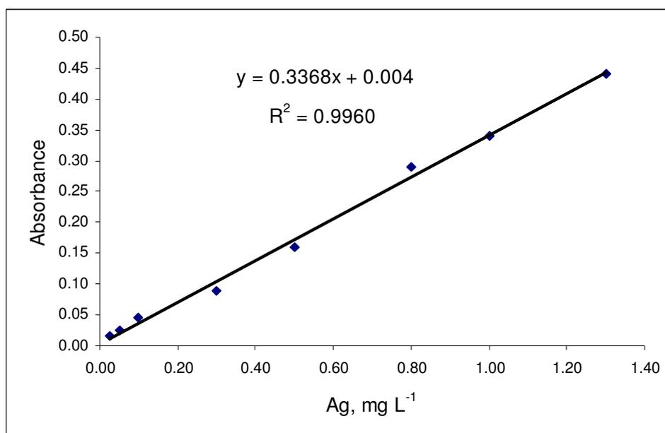
Figure 3.23 Calibration Graph for Ag Determination by CVG-FIAAS.
