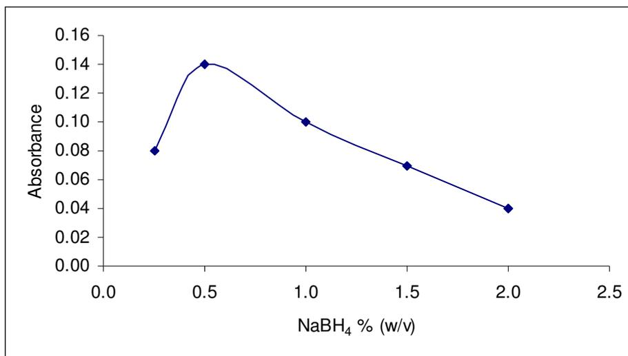
Figure 3.2 Effect of NaBH<sub>4</sub> Concentration, using 0.1 mL of 1.0 mg L<sup>-1</sup> Ag in 3.0 M HNO<sub>3</sub>, argon flow 85 mL min<sup>-1</sup>, carrier acid 1.5 M HNO<sub>3</sub>, reaction coil 4.0 cm, stripping coil 25.0 cm.
