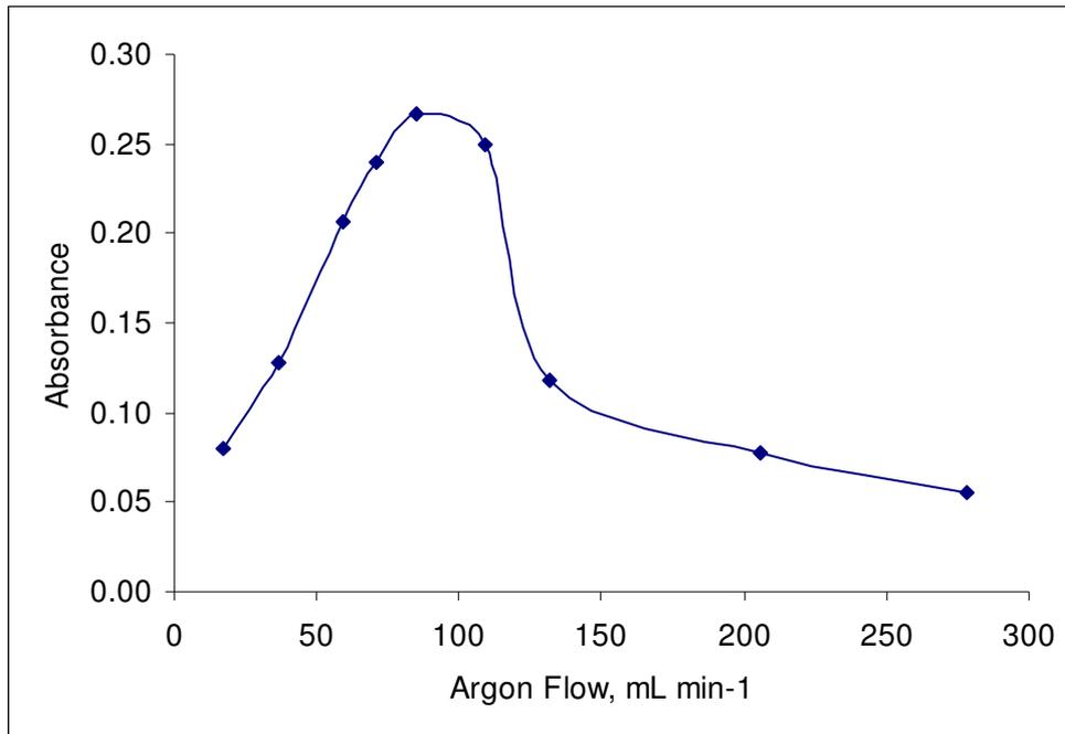
Figure 3.1 Effect of the Argon Flow Rate, using 0.2 mL of 1.0 mg L<sup>-1</sup> Ag in 3.0 M HNO<sub>3</sub>, 0.5% (w/v) NaBH<sub>4</sub> in 0.1% (w/v) NaOH, carrier acid 1.5 M HNO<sub>3</sub>, reaction coil 4.0 cm, stripping coil 25.0 cm.
