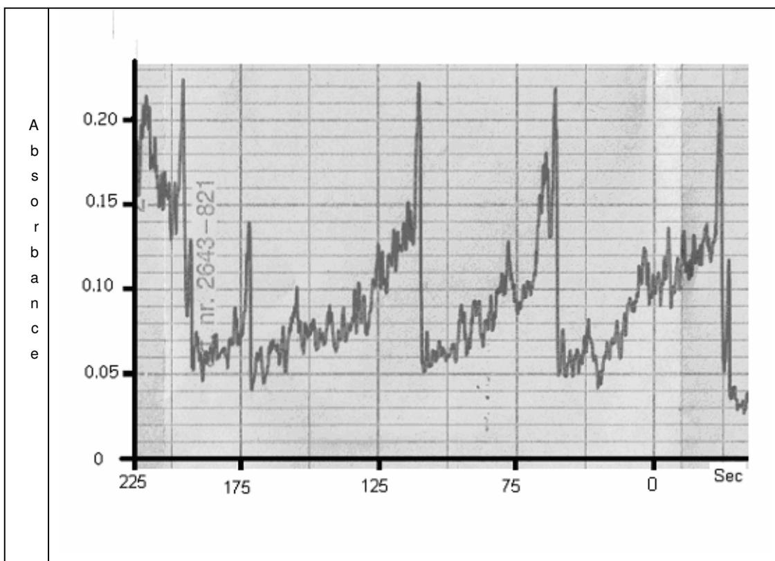
Figure 3.3 Transient Signal of Ag using 1.0 M HCl as a carrier acid with U-shaped GLS, for 0.1 mL of 1.0 mg L<sup>-1</sup> Ag in 0.6 M HCl, 0.8% (w/v) NaBH<sub>4</sub> in 0,1% (w/v) NaOH, argon flow 357 mL min<sup>-1</sup>.
