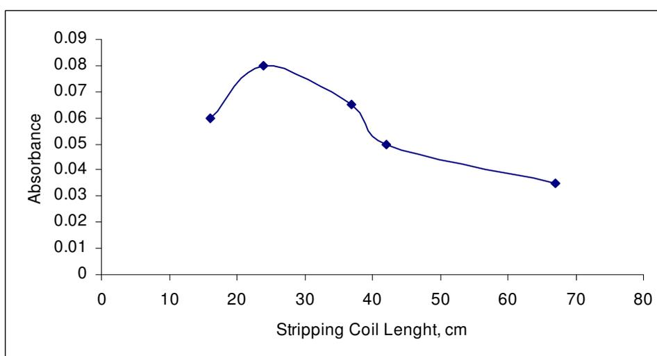
Figure 3.8 Effect of Stripping Coil Length, using 0.1 mL of 1.0 mg L<sup>-1</sup> Ag in 1.5 M HNO<sub>3</sub>, carrier acid 1.5 M HNO<sub>3</sub>, 1.0% (w/v) NaBH<sub>4</sub> in 0,1% (w/v) NaOH, argon flow 76 mL min<sup>-1</sup>, reaction coil 4.0 cm.
