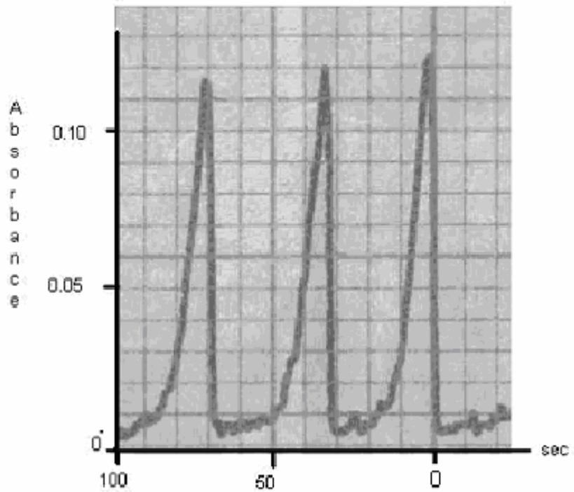
Figure 3.12 Transient Signal of CVG –AAS System Coated with 6.0 mL of 20.0 mg L<sup>-1</sup> Pd; using 0.1 mL of 1.0 mg L<sup>-1</sup> Ag in 3.0 M HNO<sub>3</sub>, carrier acid 3.0 M HNO<sub>3</sub>, 0.5% (w/v) NaBH<sub>4</sub> in 0,1% (w/v) NaOH, argon flow 85 mL min<sup>-1</sup>, reaction coil 4.0 cm, stripping coil 25.0 cm.
