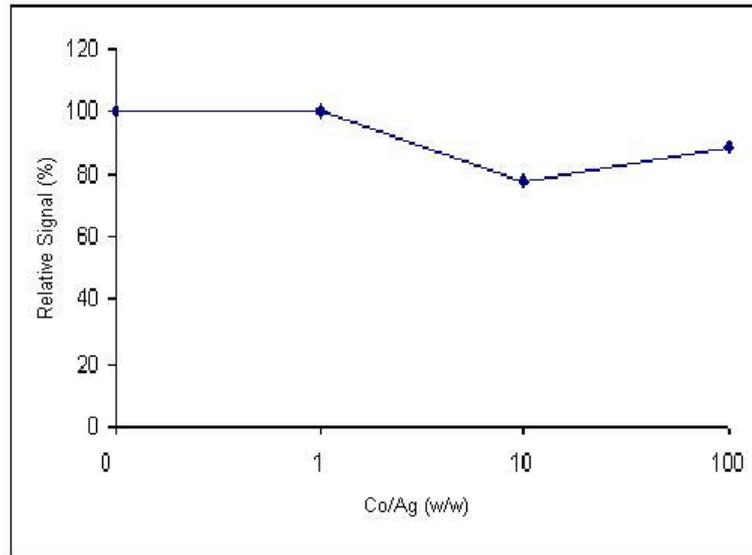
Figure 3.16 Interference of Cobalt on Ag CVG Signal
