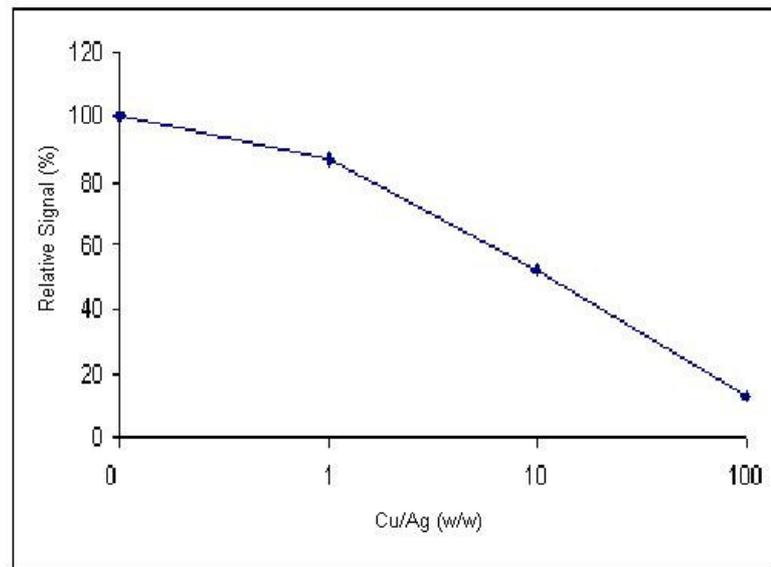
Figure 3.15 Interference of Copper on Ag CVG Signal
