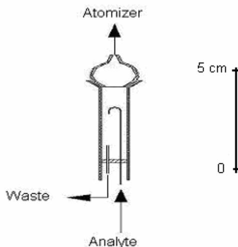
Figure 2.2 Cylindrical Gas- Liquid Separator Design
