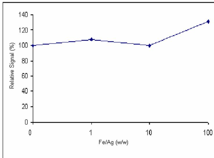
Figure 3.17 Interference of Iron on Ag CVG Signal
