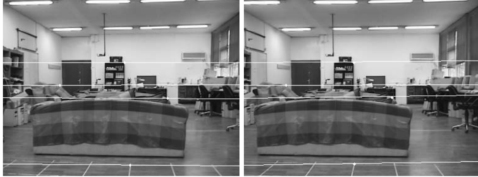
Figure 3.6: Two views taken from a nearly parallel cameras. Corresponding point of an image point in one view lies on the corresponding epipolar line. Note that epipolar lines are almost parallel.
