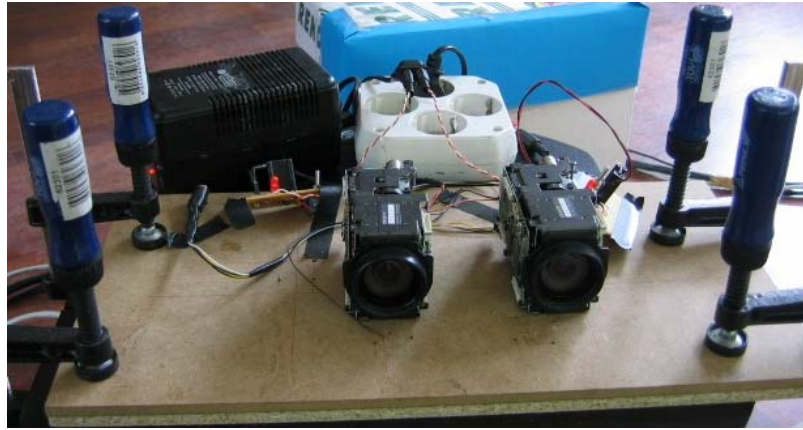
Figure 4.2: Camera system is developed in the laboratory and consists of two Sony board cameras.
