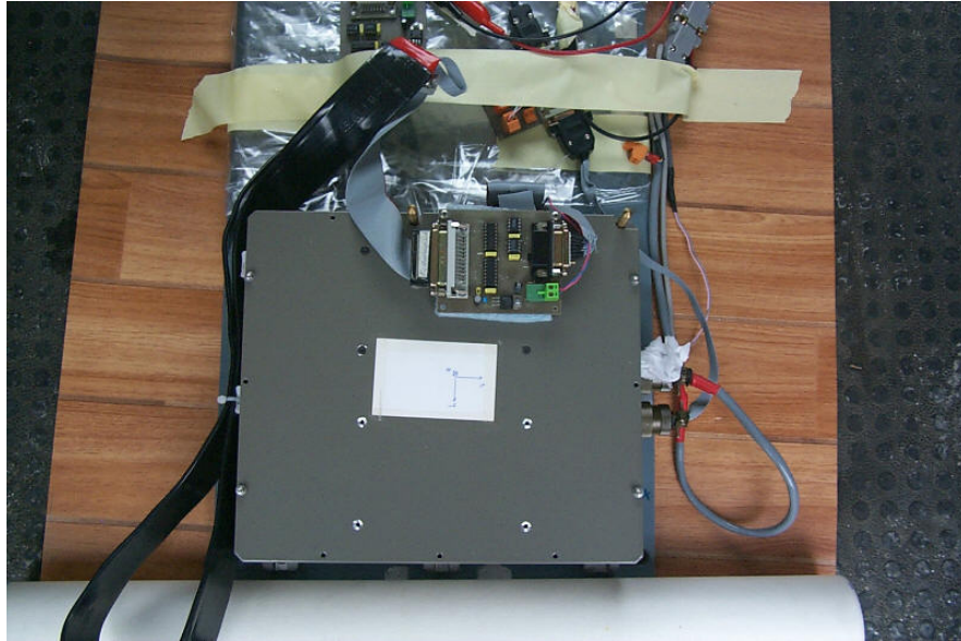
Figure 2-16 GPS/INS system mounted on the test vehicle for navigation purposes and real time data collection.
