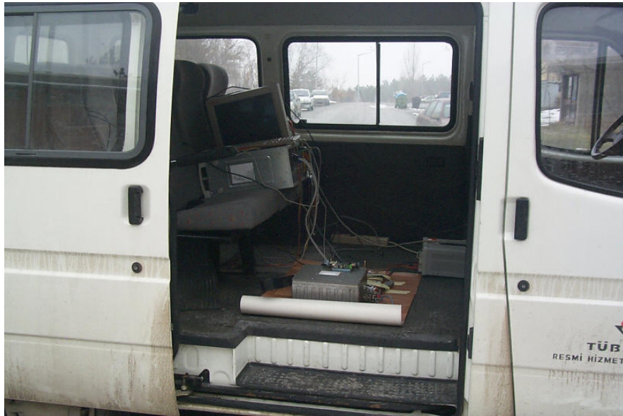
Figure 2-14 The van is used as a test vehicle for GPS/INS system. It contains the GPS antenna and GPS/INS unit. It also houses laptop and desktop computers for monitoring and real time data collection.
