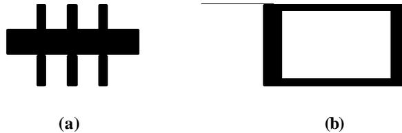
Fig.3. 1: a) Six arm-bridge (Hall bar), and b) Mask geometry for structural measurements of film studies.
