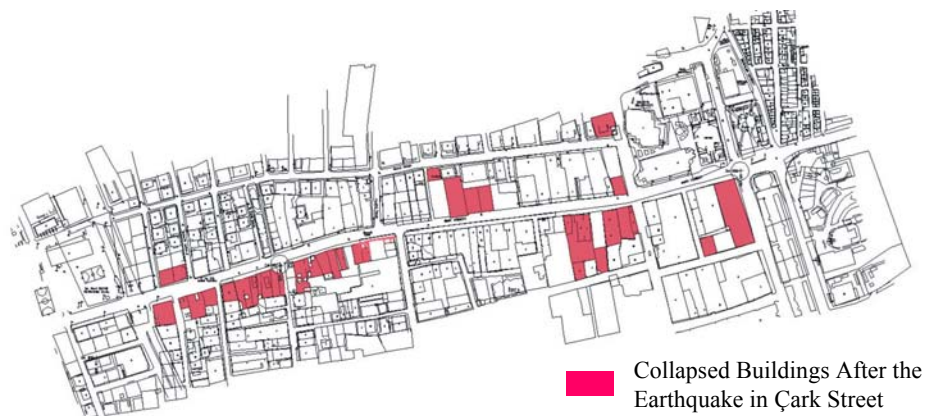
Figure 5.12: Collapsed Buildings After the Earthquake in Çark Street
