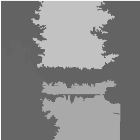
Figure 4.32: Segmentation of test image 2 with RSST with Region Intensity Modeling by texture.
