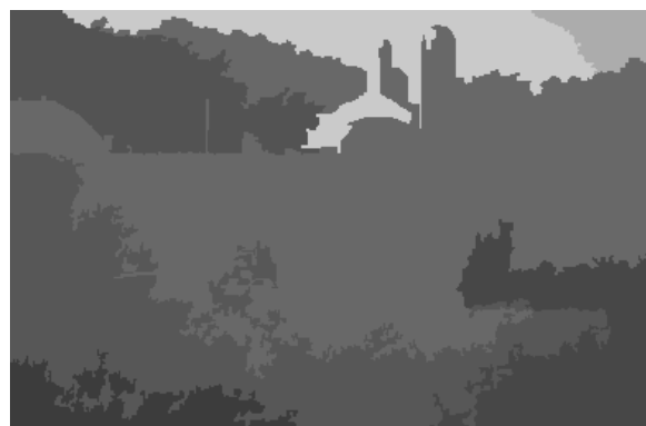
Figure 4.23: Segmentation of test image 7 with RSST with Region Intensity Modeling by histogram.
