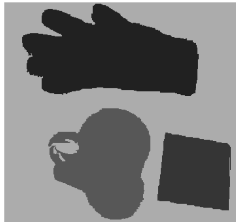
Figure 4.20: Segmentation of test image 3 with RSST with Region Intensity Modeling by histogram.
