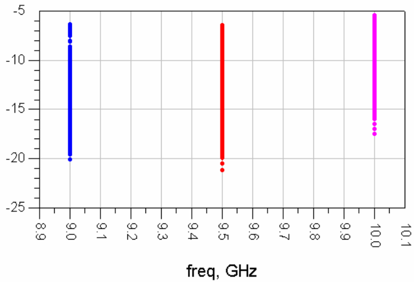
Figure 6.7 Insertion loss of the vector modulator in polar coordinate at 10 GHz (Dynamic Range of -38dB to -2 dB)
