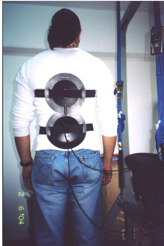
Figure 3.5. The placement of the accelerometers in accordance with anatomical reference points
