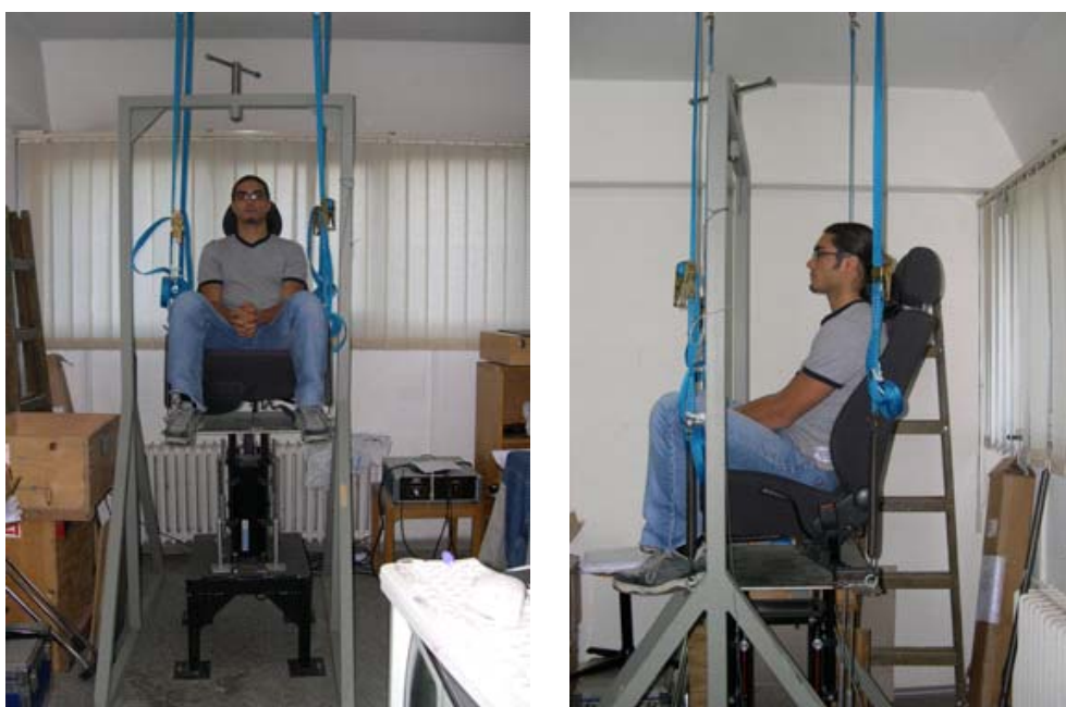
Figure 3.2 The laboratory setup of the seat on the shaker table.
