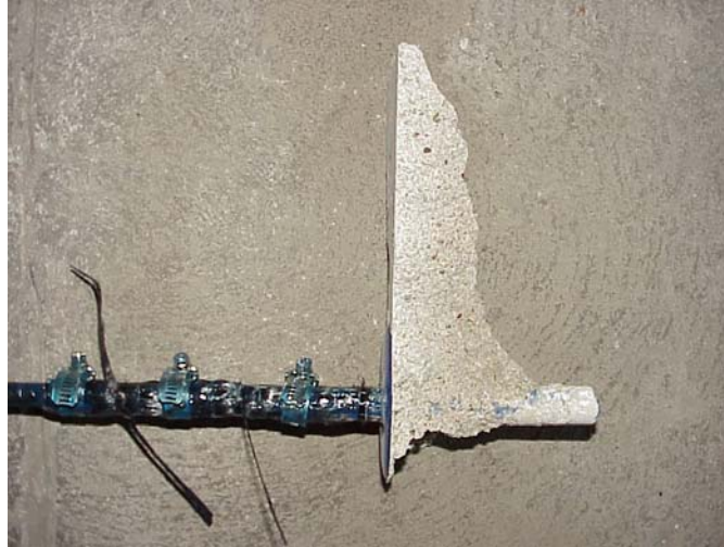
Figure 3.6 Side view of the failed CFRP anchor dowel
