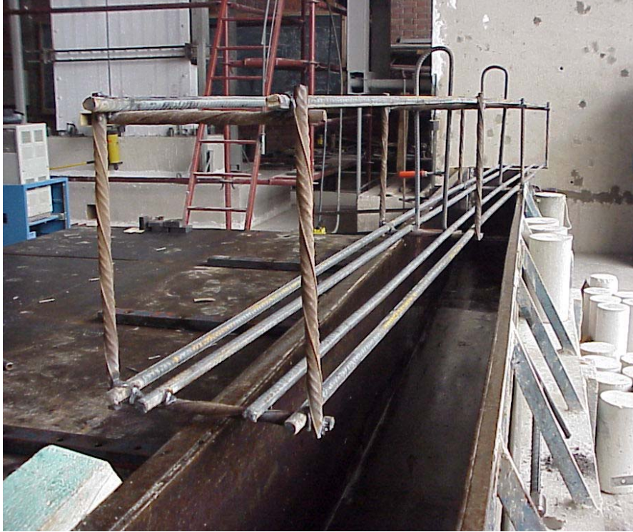
Figure 2.3 Reinforcement detail of the beam
