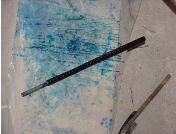
Figure 2.8 CFRP sheet is bonded to either of the steel or silicon rods
