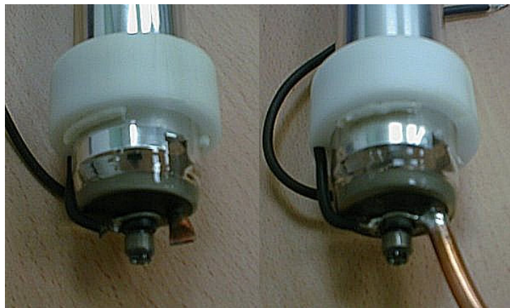
Figure 3.3: Tube end, before and after soldering.
