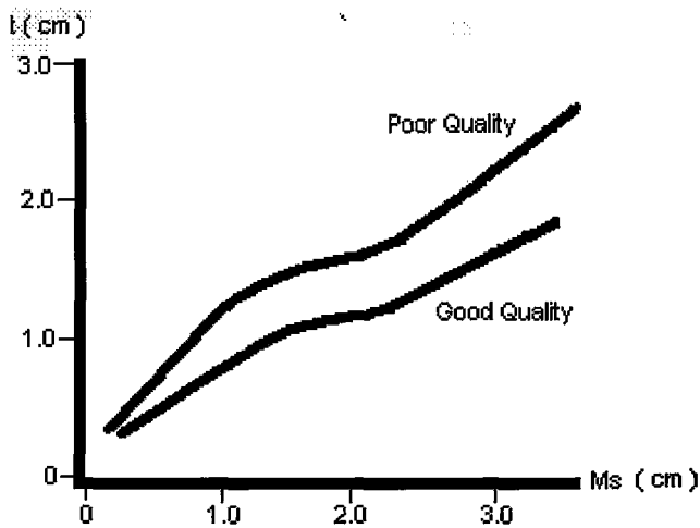
Figure 4. Transfer modulus vs. significant modulus as a function of metallurgical quality. [ 5 ]
