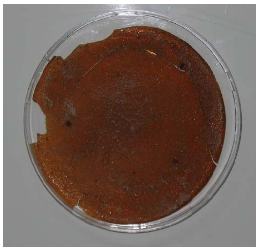
Figure 3.4 Photograph of 10% (w/w) birchwood xylan film prepared by using the washing solution left after the xylan extraction.
