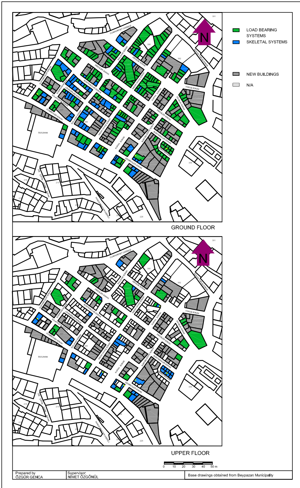
Figure 17 Structural systems - ground floors
