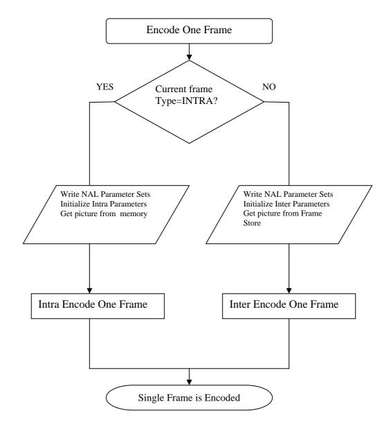
Figure 18 - Encode One Frame flow chart
