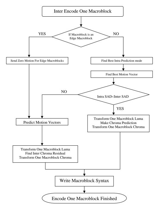
Figure 21 - Inter Encode One Macroblock flow chart
