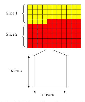
Figure 4 - Sample QCIF frame with two slices showing single luminance macroblock
