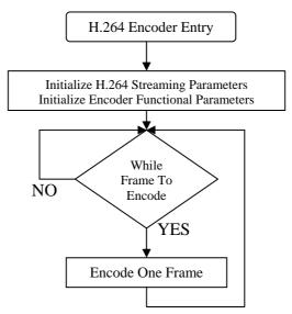
Figure 17 - Main loop flowchart
