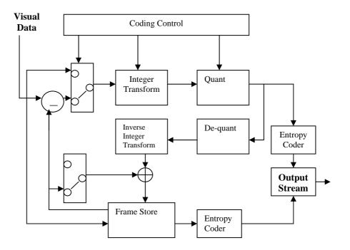
Figure 16 - H.264 Encoder block diagram
