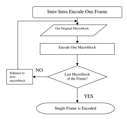
Figure 19 - Inter-Intra Encode One Frame flow chart
