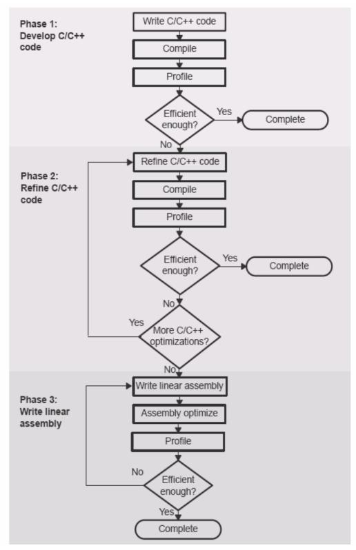
Figure 24 – Code development cycle for TMS320C64x [27]
