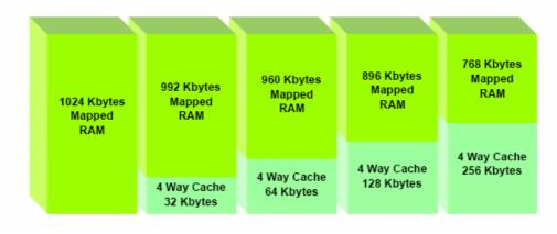
Figure 14 – C64x internal memory architecture [8]
