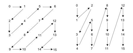
Figure 10 - Coefficient scan patterns for Zig-zag Scan and Field Scan [7]
