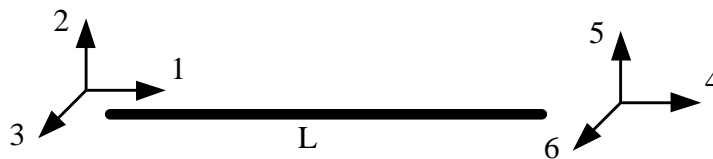
Figure 3.6: 3 dimensional, 2 node truss element
