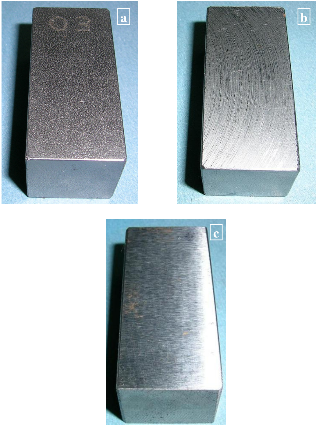
Figure 5.4 Surface conditions of specimens a) raw, b) milled and c) ground
