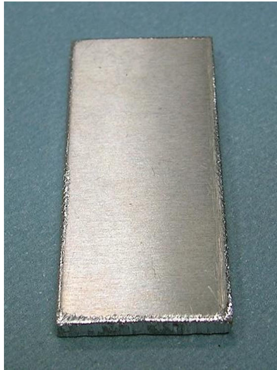
Figure 5.6 An Al5086 specimen
