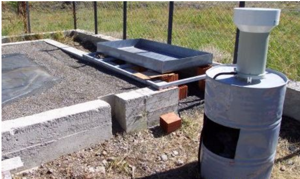
Figure 3.13 Snowmelt lysimeter and rain-gauge in Güzelyayla station
