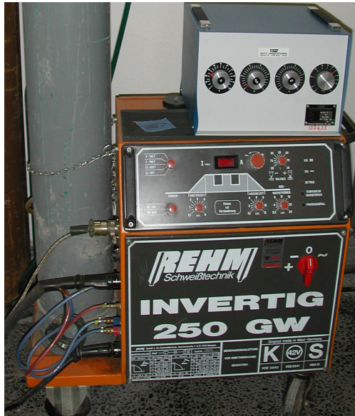
Figure 3.6: Welding power supply and the gas mixer.
