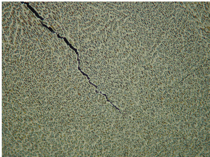
Figure 4.70: Weld metal surface microstructure before the bending point. Type “A” crack inside fine solidification structure. TIG-DC welded specimen. Line energy: 2.3 kJ/cm; Augmented strain: 1.0 %. Weck etching. 200X magnification.
