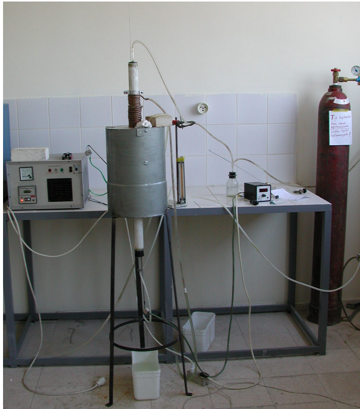
Figure 3.8: Vertical furnace used for the quench tests.
