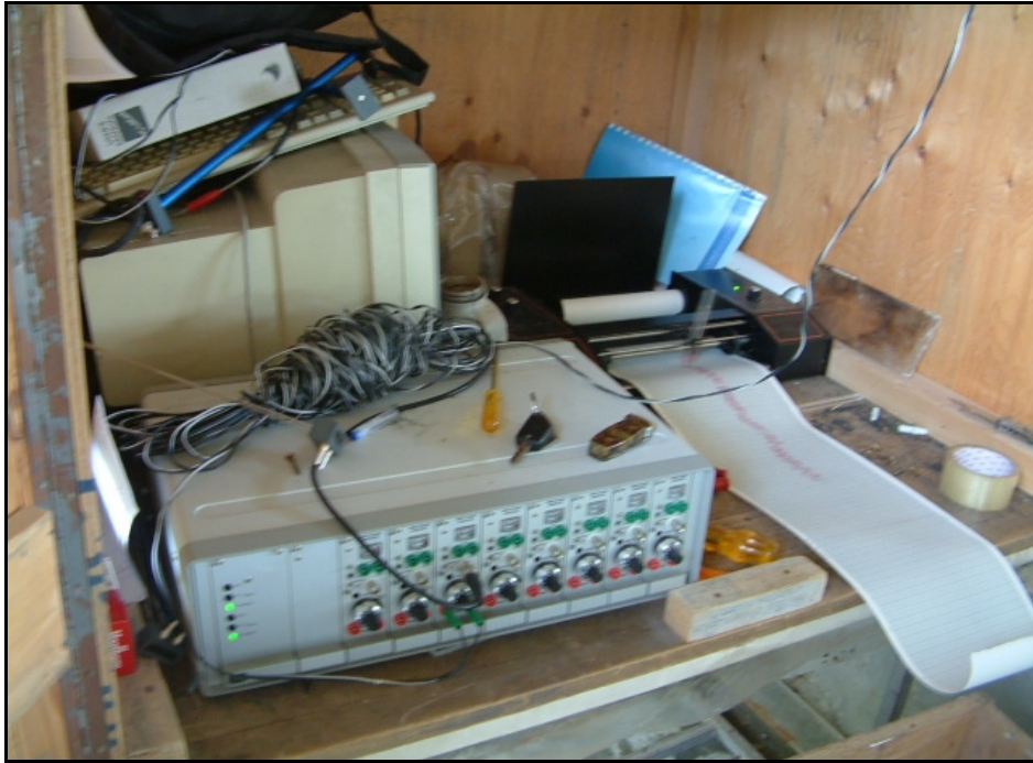
Figure 3.6: View of Wave Probe Monitor and Plotter
