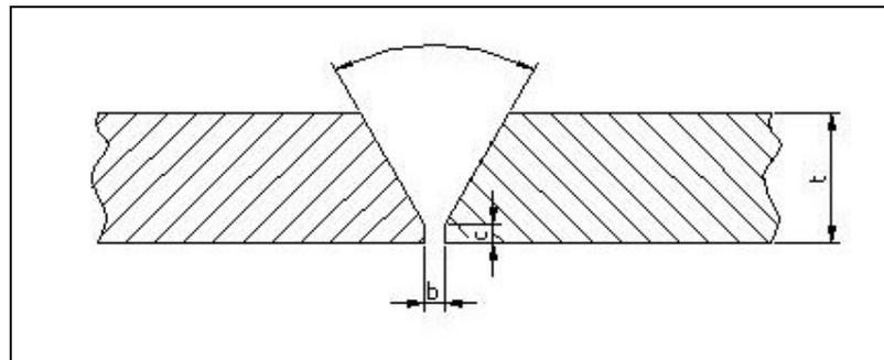
Fig. 2.1: Dimensions of V shaped weld seam
