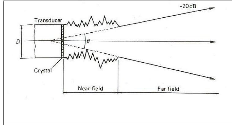
Fig 4.2: Profile of an Ultrasonic Beam
