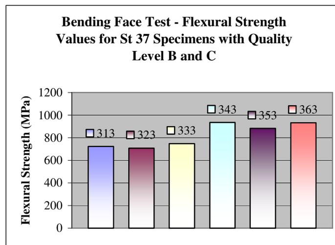
Fig. 7.27: Bending Face Test – Flexural Strength Values for St 37 Specimens with Quality Level B and C
