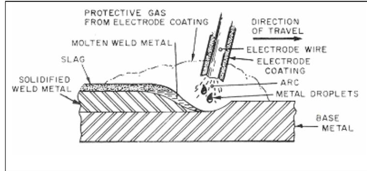
Fig. 2.2: Shielded Metal Arc Welding
