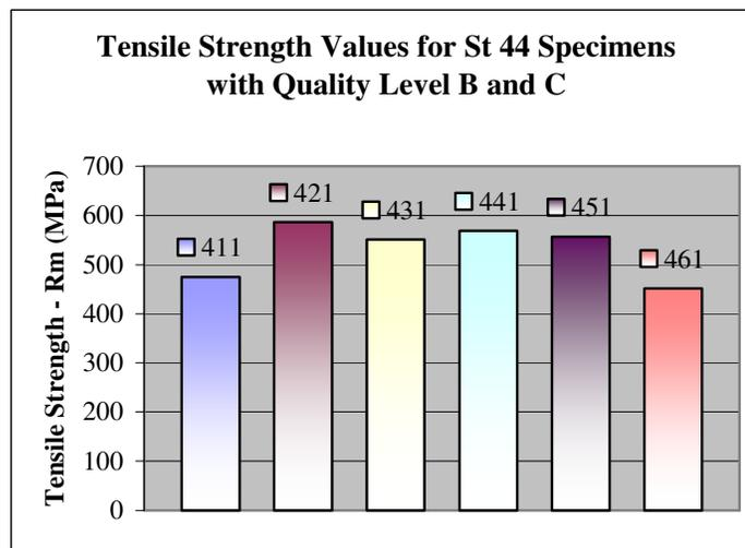
Fig. 7.19: Tensile Strength Values for St 44 Specimens with Quality Level B and C
