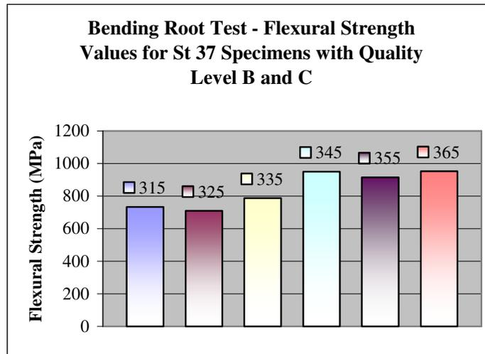
Fig. 7.30: Bending Root Test – Flexural Strength Values for St 37 Specimens with Quality Level B and C
