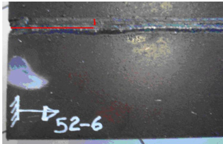
Fig 7.4: Reference Point for Radiographic Examination
