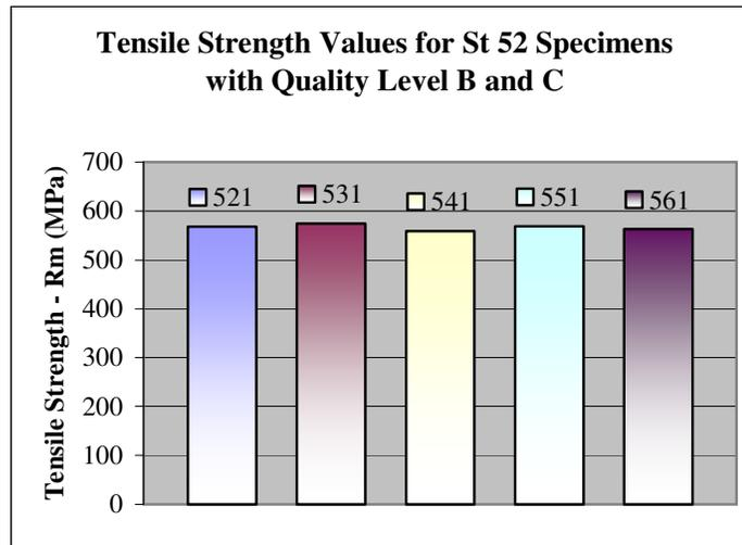
Fig. 7.20: Tensile Strength Values for St 52 Specimens with Quality Level B and C
