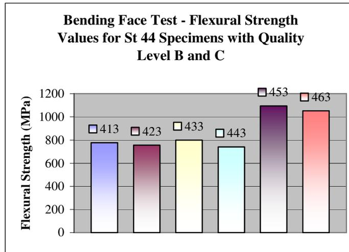
Fig. 7.28: Bending Face Test – Flexural Strength Values for St 44 Specimens with Quality Level B and C
