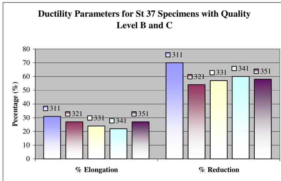
Fig. 7.24: Ductility Parameters for St 37 Specimens with Quality Level B and C
