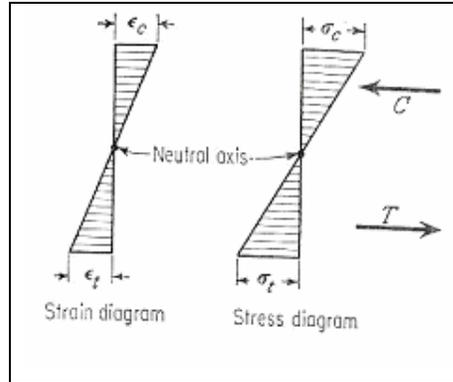
Fig. 6.3: Strain and Stress Diagrams
