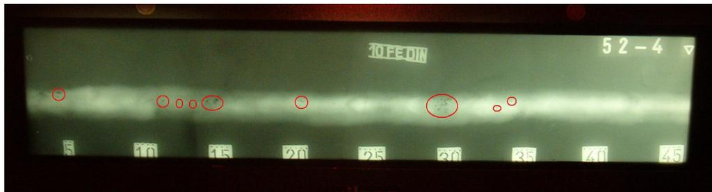
Fig.7.6: Radiographic Film of Quality Level C
