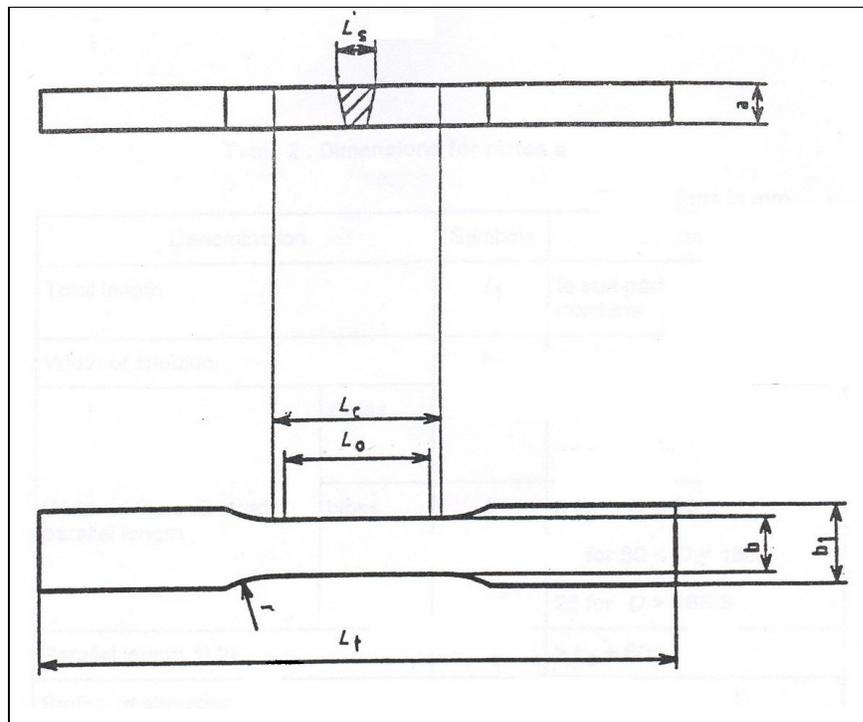
Fig. 5.5: Tensile Test Specimen for Plates
