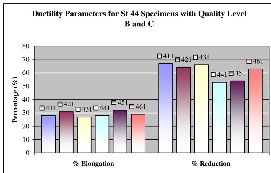
Fig. 7.25: Ductility Parameters for St 44 Specimens with Quality Level B and C
