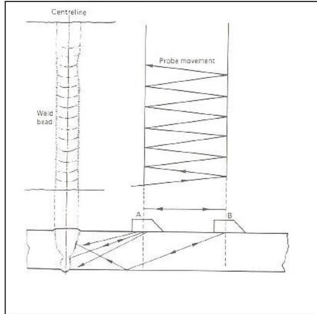
Fig. 4.4: Ultrasonic Scan Path
