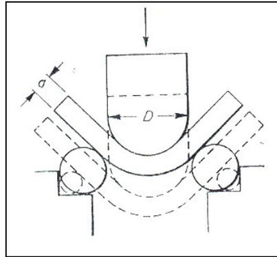
Fig. 6.7: Bending Test Arrangement
