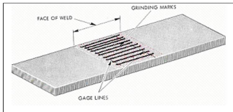
Fig. 6.9: Free-Bend Test
