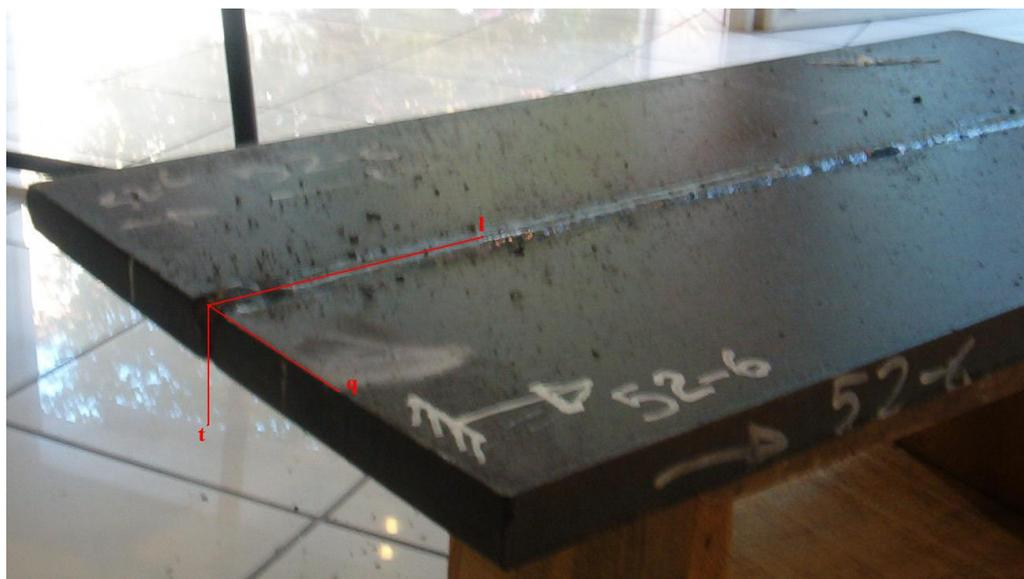
Fig. 7.13: Reference point for Ultrasonic Examination
