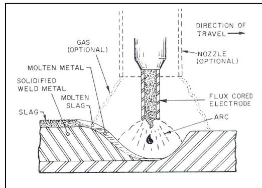
Fig. 2.7: Flux-Cored Arc Welding
