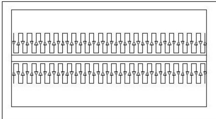
Fig. 7.12: Prop Movement for Ultrasonic Testing
