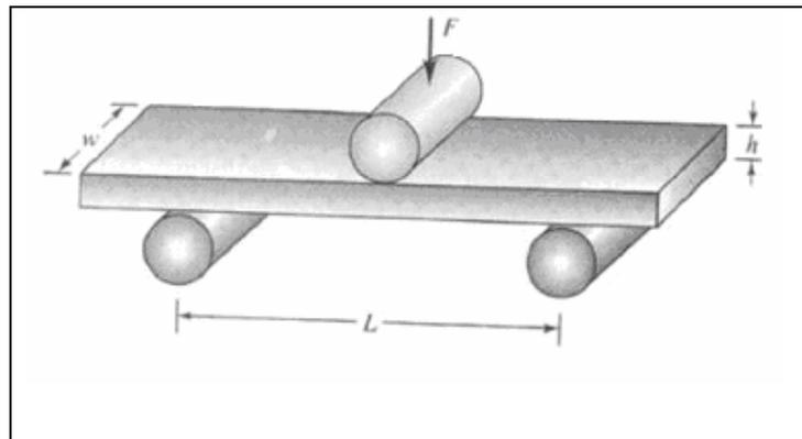
Fig. 6.5: Three-Point Bending
