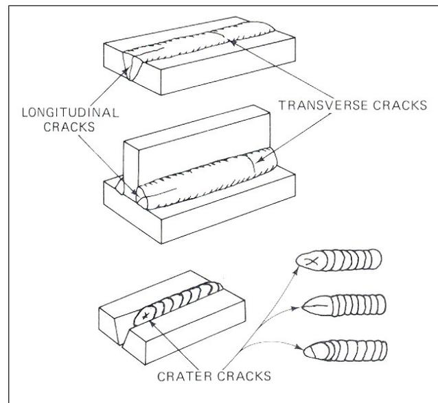
Fig. 2.9: Surface Cracks
