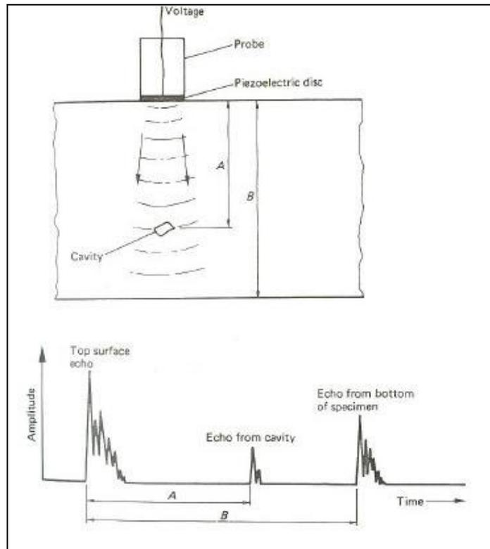
Fig. 4.1: Application of Ultrasonic Flaw Detection
