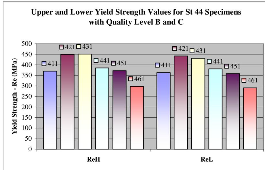
Fig. 7.22: Upper and Lower Yield Strength Values for St 44 Specimens with Quality Level B and C
