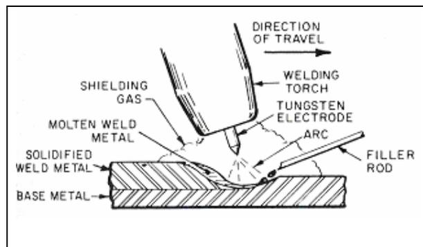
Fig. 2.3: Gas Tungsten Arc Welding
