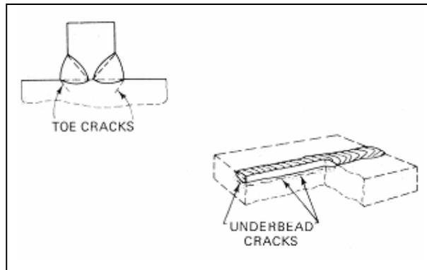
Fig. 2.10: Subsurface Cracks
