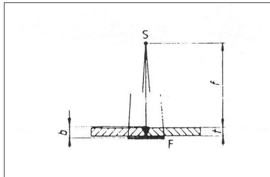
Fig. 7.3: Radiographic Test Arrangement
