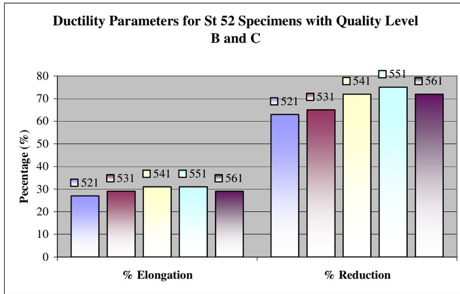
Fig. 7.26: Ductility Parameters for St 52 Specimens with Quality Level B and C
