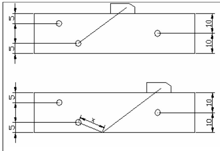
Fig. 7.10: Direct and Indirect Sound Attenuation
