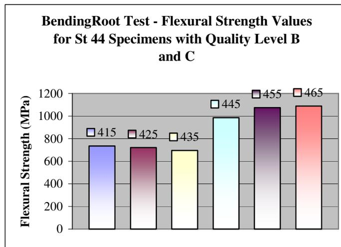
Fig. 7.31: Bending Root Test – Flexural Strength Values for St 44 Specimens with Quality Level B and C
