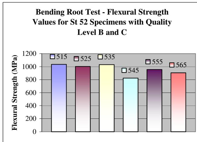
Fig. 7.32: Bending Root Test – Flexural Strength Values for St 52 Specimens with Quality Level B and C
