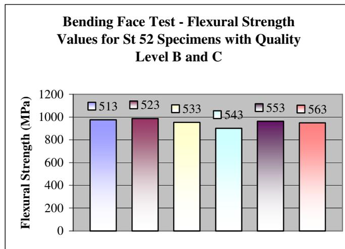
Fig. 7.29: Bending Face Test – Flexural Strength Values for St 52 Specimens with Quality Level B and C
