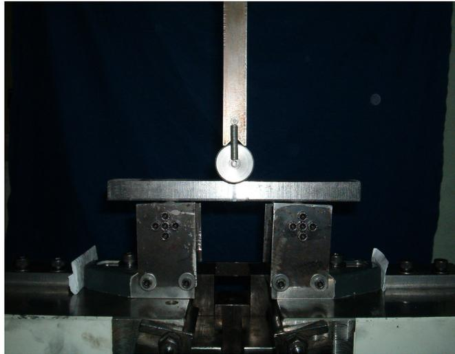
Fig. 7.16: Bending Test Apparatus
