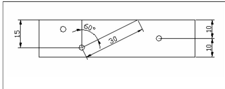
Fig. 7.7: Drilled Part Used for DGS Curve Sensitivity Setting
