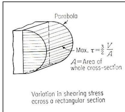
Fig. 6.4: Shearing Stress at Rectangular Section
