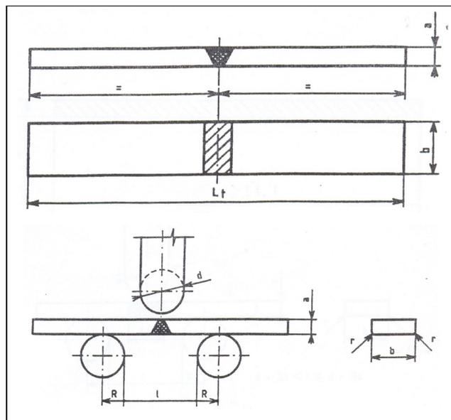
Fig. 6.10: Bending Test Specimen
