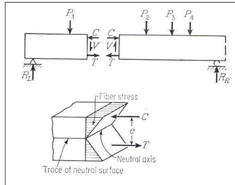
Fig. 6.1: Beam Subjected to Transverse Loading
