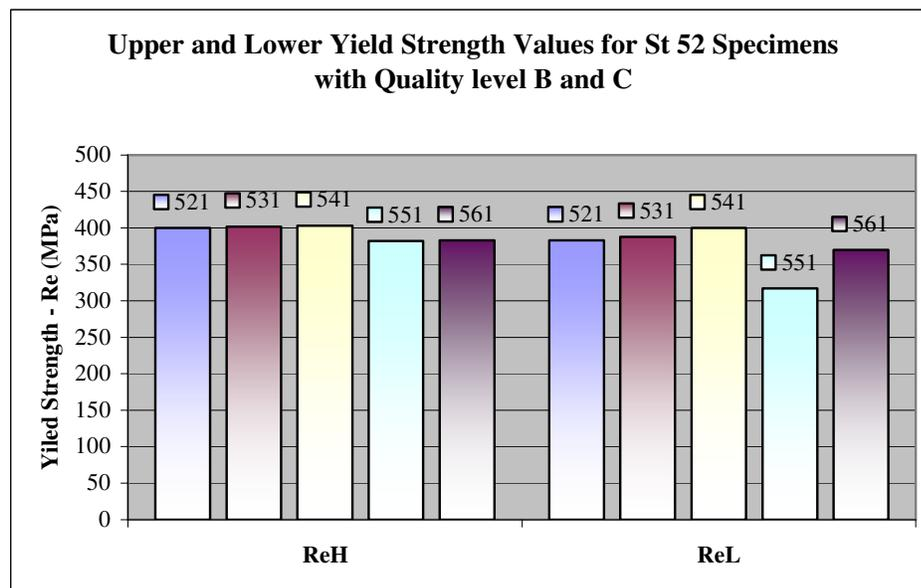
Fig. 7.23: Upper and Lower Yield Strength Values for St 52 Specimens with Quality Level B and C
