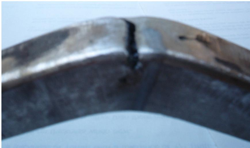
Fig. 8.2: Bending Specimen Fractured at Low  $F_m$
