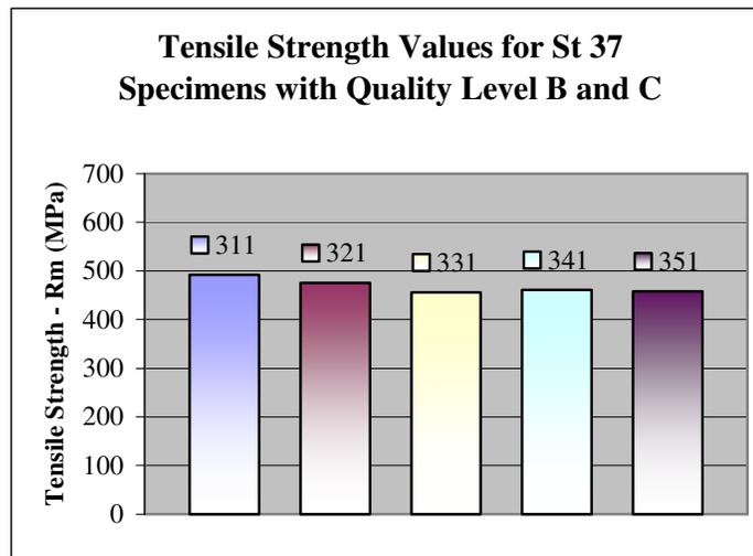
Fig. 7.18: Tensile Strength Values for St 37 Specimens with Quality Level B and C
