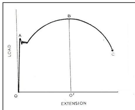
Fig. 5.1: Load-elongation Curve
