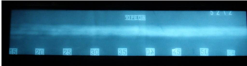
Fig.7.5: Radiographic Film of Quality Level B
