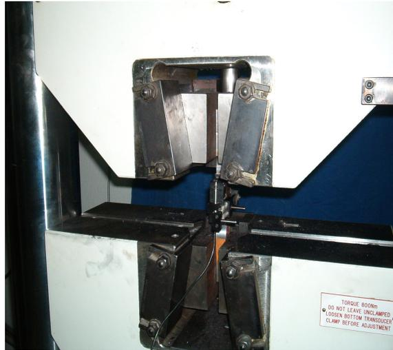
Fig 7.15: Tensile Test Apparatus
