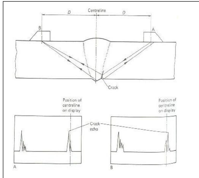
Fig. 4.3: Root Crack
