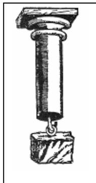
Fig. 5.4: Galileo's Tensile Test Apparatus
