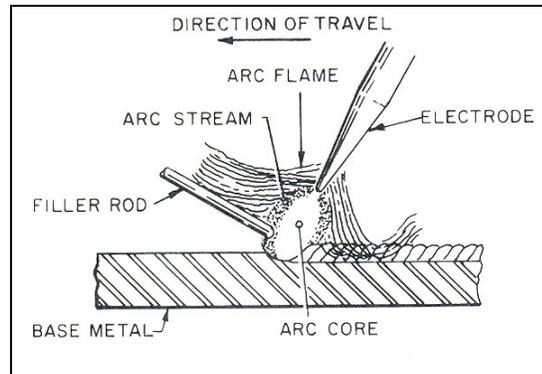
Fig. 2.5: Carbon Arc Welding
