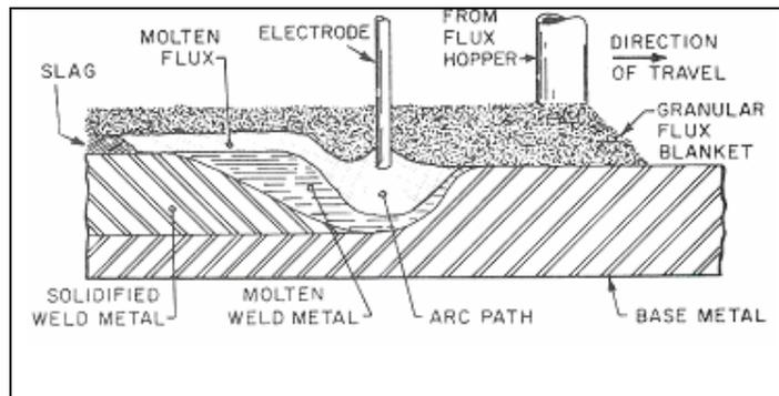
Fig. 2.6: Submerged Arc Welding
