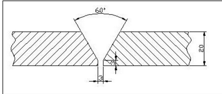
Fig.7.1: V Shaped Welding
