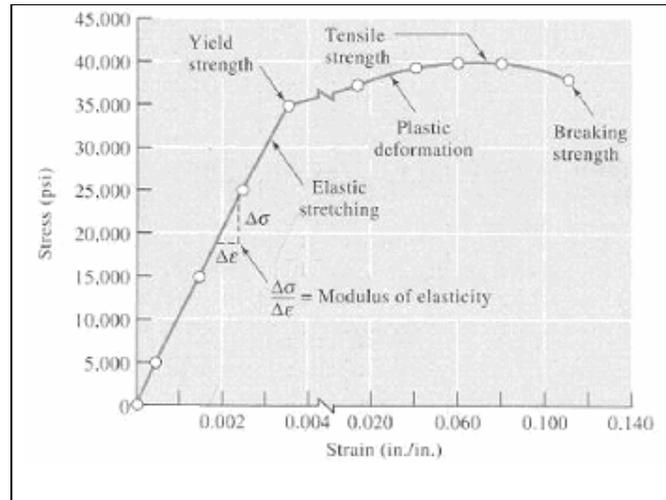
Fig. 5.2: Stress-Strain Curve
