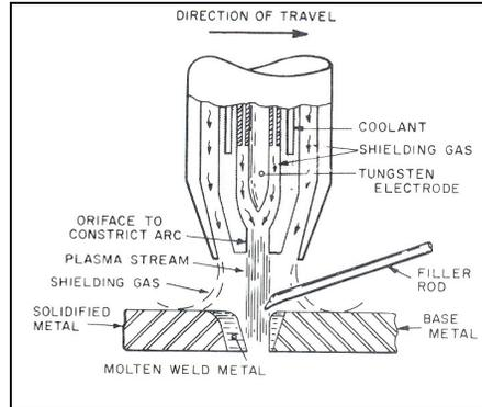
Fig. 2.4: Plasma Arc Welding
