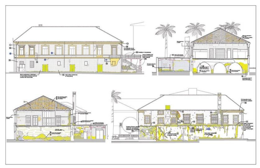
Drawing 2.35 Analysis on Material Deteriorations and Structural Deformations
