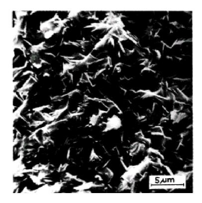
Figure 4.14 SEM micrograph of the machinable glass ceramic with flat, flakelike, fluorphlogopite crystals given by Vogel et al.[25].
