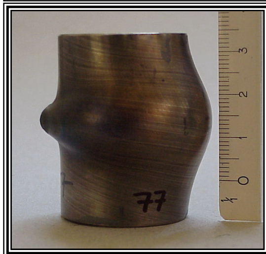
Experiment 77 Voltage: 475 V Energy: 3.5 J/Pulse
