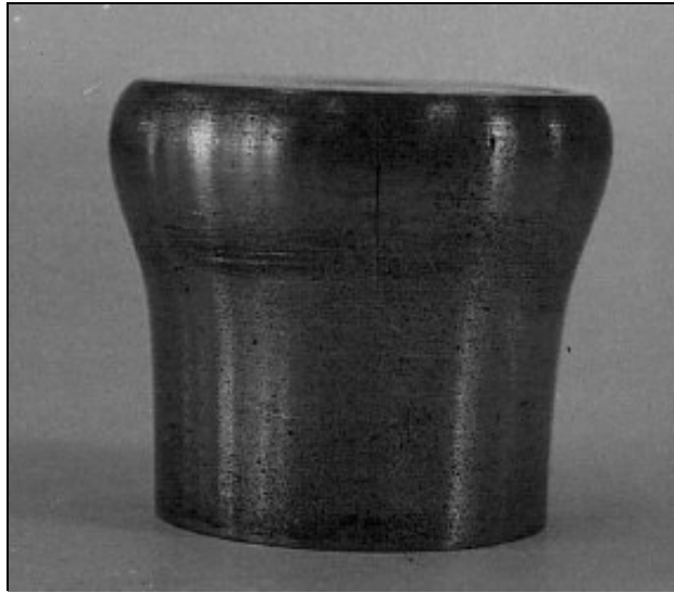
Figure 2.10 Part produced with induction heating
