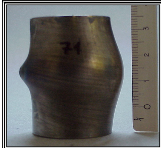
Experiment 71 Voltage: 450 V Energy: 3.1 J/Pulse
