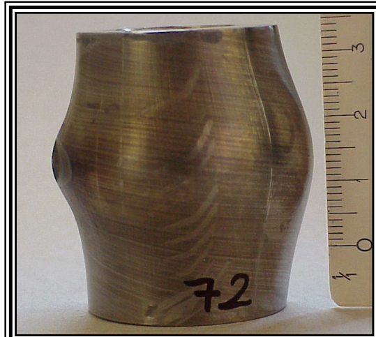
Experiment 72 Voltage: 400 V Energy: 2.1 J/Pulse
