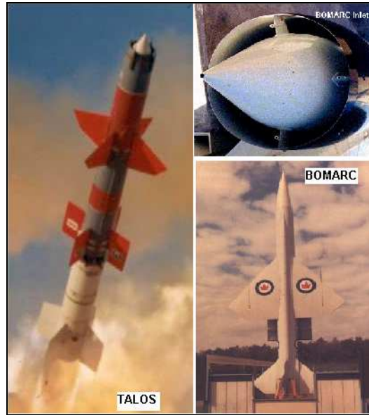
Figure 3.7 Surface-to-air ramjet missiles and their inlets
