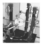
Figure 2.10 Modular Parallel Robot [27].
