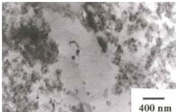
Figure 2.6. TEM micrograph of the microstructure of the extrudate produced from coarse powder particles [22]
