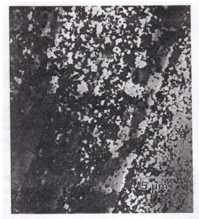
Figure 2.9. Microstructure of extruded samples of FVS1212 alloy after annealing 500h at 550°C. [21]
