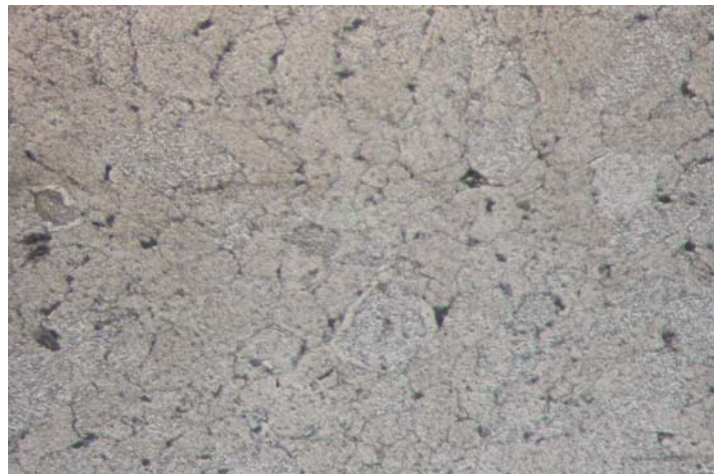
Fig. 2.21a) The development of the interparticle bond during sintering, starting with a point contact. The pore volume shrinks and the pores become smoother. As pore sinterodization occurs, the pores are replaced with grain boundaries. [14] b) sintered product with pores at powder boundaries.
