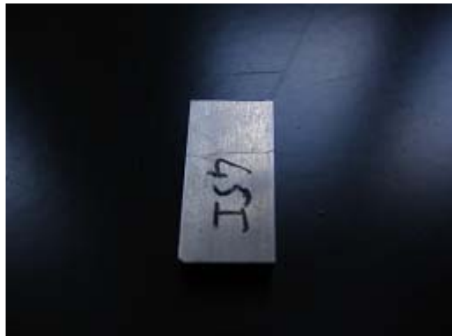
Figure 4.1 Photography of the specimen with a delamination crack
