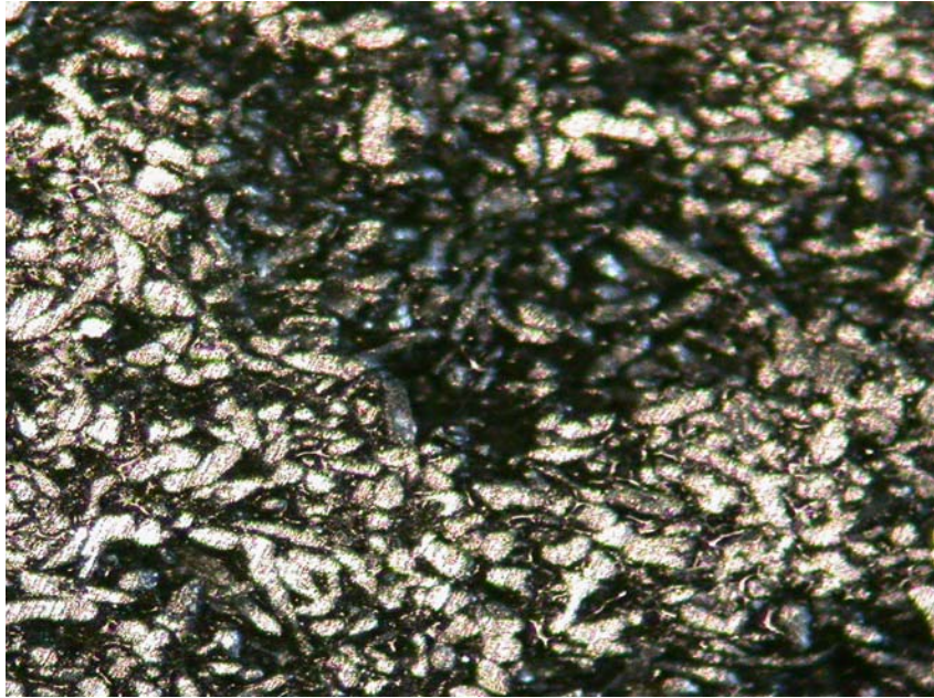
Figure 4.37 Optical micrograph of the alloy powder of +53 \mu m ( X50)
