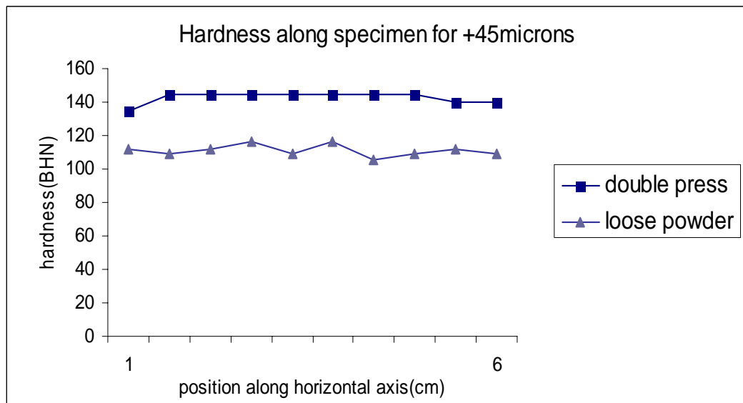
Figure 4.8. Hardness along specimen which were produced from +45 \mu m alloy powder
