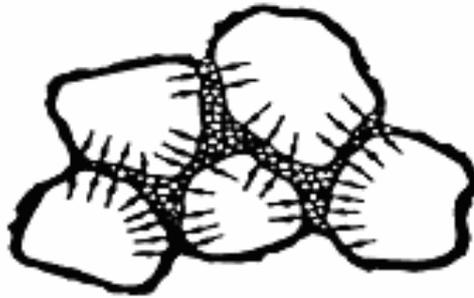
**Figure 2.2.** Structure of Collapsible Soils (Loaded Structure after Inundation)
