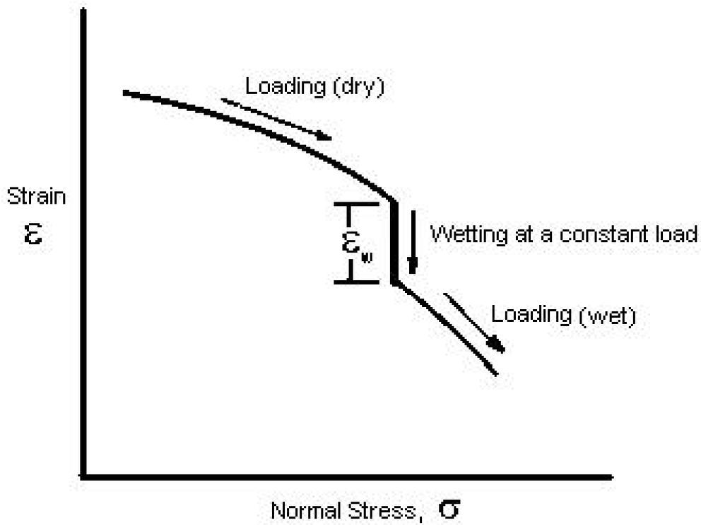
**Figure 2.4.** Single Oedometer Test Results (Houston, et al., 1988)
