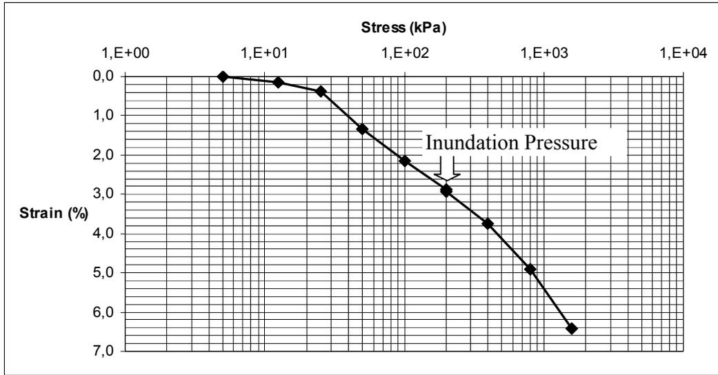
**Figure A.7.** Consolidation Test Result of 25% FA
