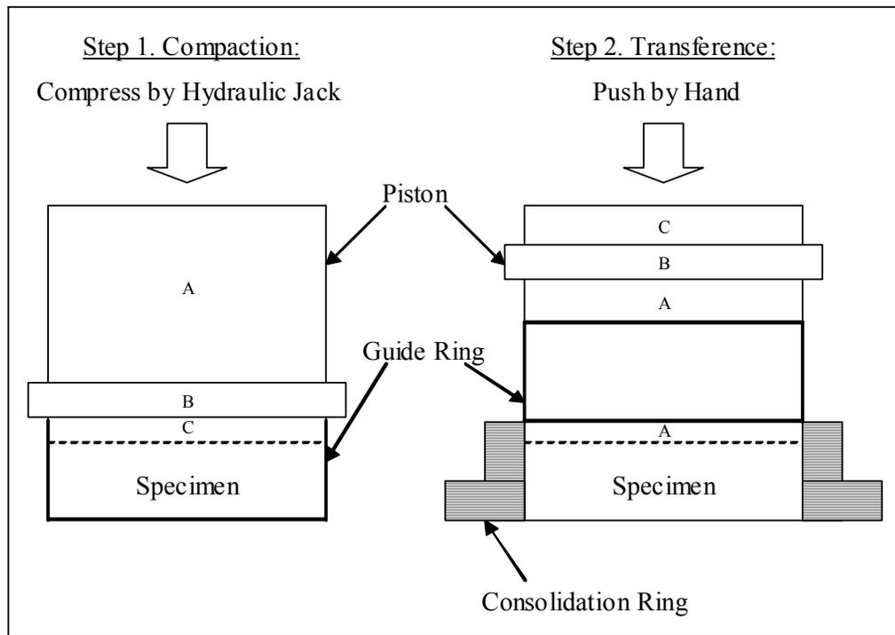
**Figure 4.5.** Static Compaction Setup (Çetiner, 2004)
