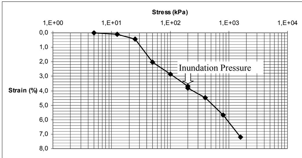
**Figure A.5.** Consolidation Test Result of 15% FA
