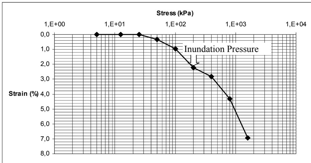
**Figure A.6.** Consolidation Test Result of 20% FA
