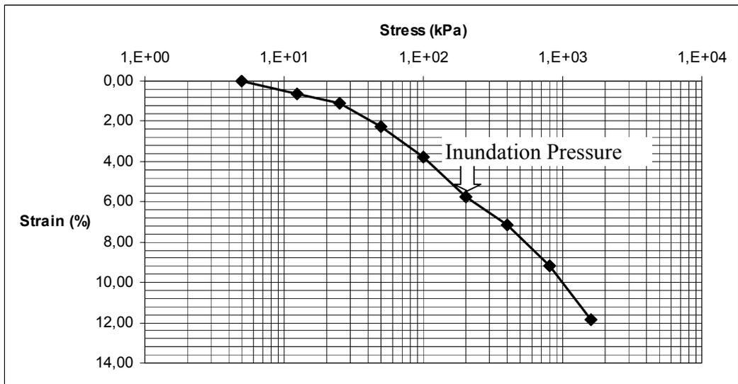
**Figure A.2.** Consolidation Test Result of 100% A Compacted
