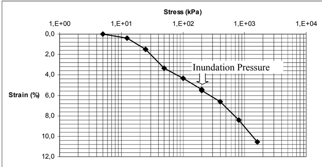
**Figure A.3.** Consolidation Test Result of 5% FA
