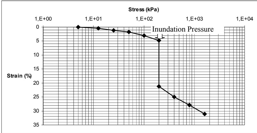
**Figure A.1.** Consolidation Test Result of 100% A Undisturbed
