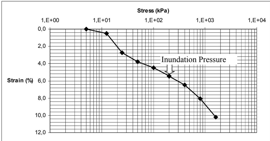
**Figure A.8.** Consolidation Test Result of 5% DSG
