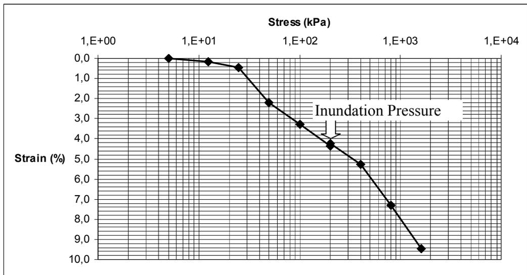
**Figure A.10.** Consolidation Test Result of 15% DSG
