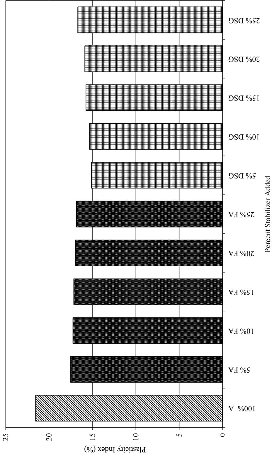
**Figure 4.10.** Effects of Addition of Fly Ash and Desulphogypsum on the Plasticity Index
