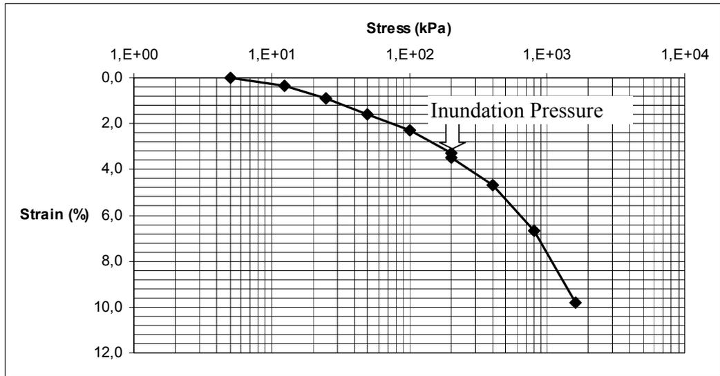
**Figure A.9.** Consolidation Test Result of 10% DSG
