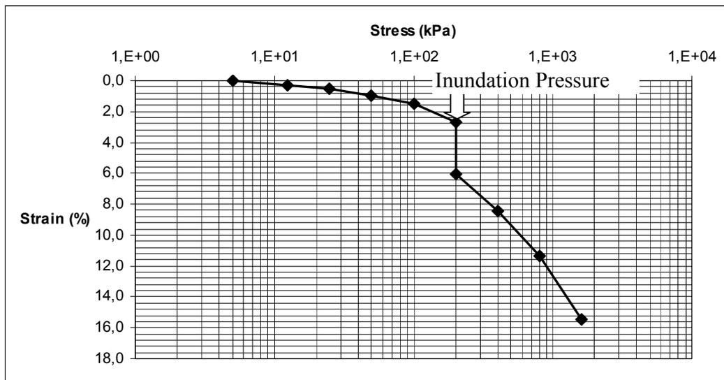
**Figure A.12.** Consolidation Test Result of 25% DSG
