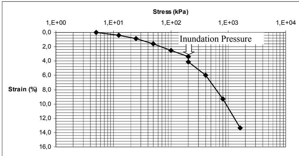
**Figure A.11.** Consolidation Test Result of 20% DSG
