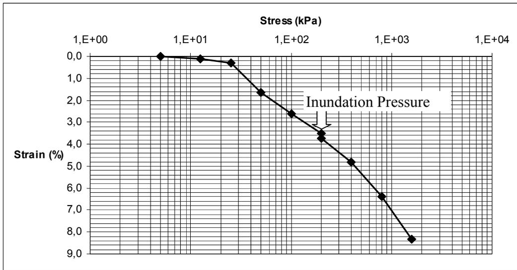
**Figure A.4.** Consolidation Test Result of 10% FA
