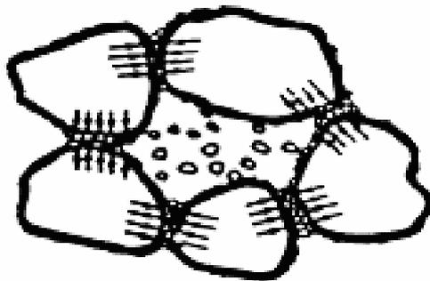
**Figure 2.1.** Structure of Collapsible Soils (Loaded Structure before Inundation)
