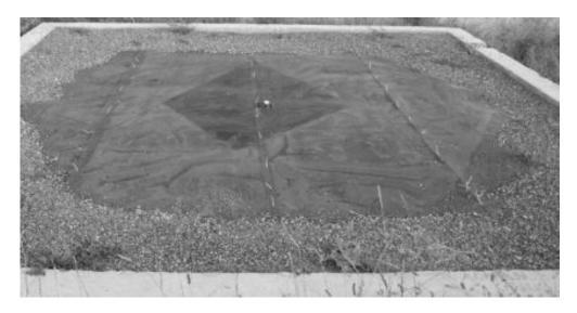
Figure 2.10 Installed snow pillow at Güzelyayla station
