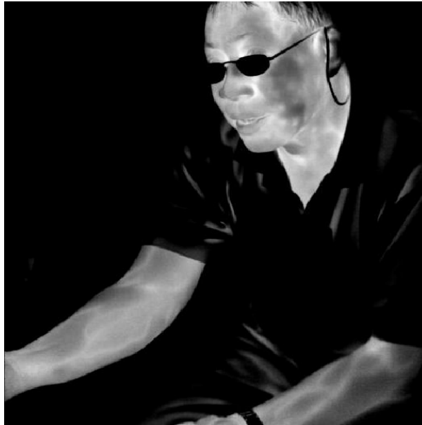
Figure 2.6: An example image taken with 1024×1024 MWIR QWIP camera developed by JPL in collaboration with U.S. Missile Defense Agency and U.S. Air Force Research Laboratory [69].
