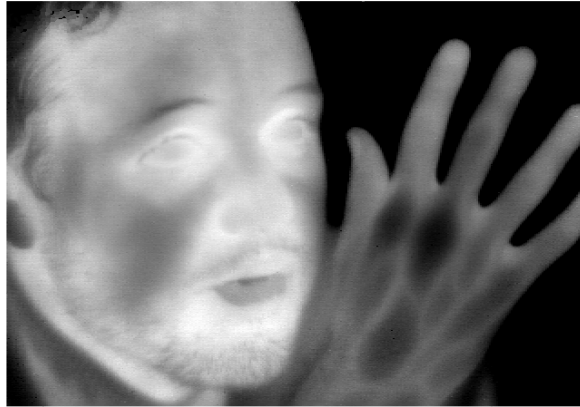
Figure 7.9: Indoor thermal image taken with the InP/InGaAs QWIP FPA at 70 K sensor temperature [169].
