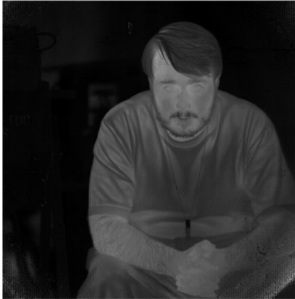
Figure 2.7: Image taken with the 1K×1K LWIR QWIP camera developed at JPL [72].
