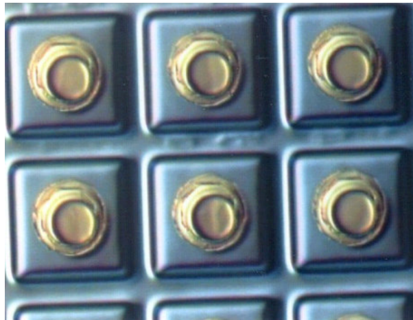
Figure 3.29: Optical microscope picture of the FPA pixels after UBM deposition.
