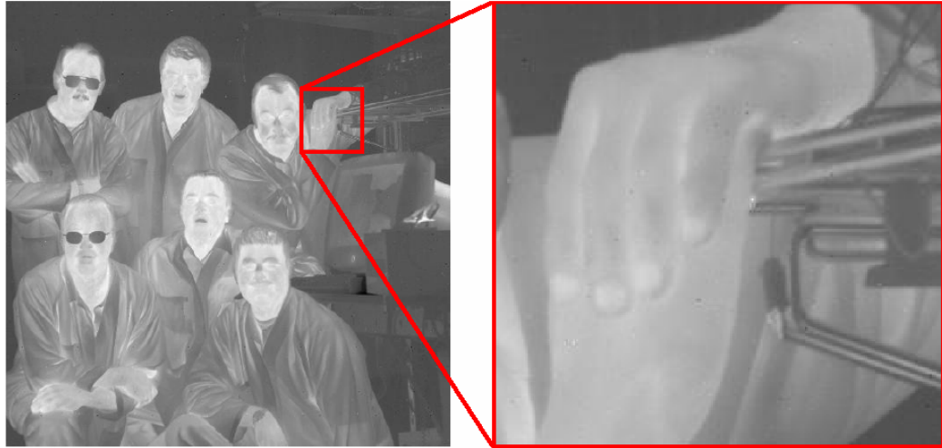
Figure 2.3: Images from 2\text{K}\times 2\text{K} InSb FPA produced by CMC Electronics Cincinnati. The magnified portion of the image shows the resolution of the FPA [40].
