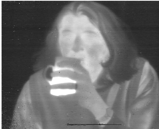
Figure 5.18: A snapshot from 640×512 MOCVD grown AlGaAs/GaAs QWIP FPA.
