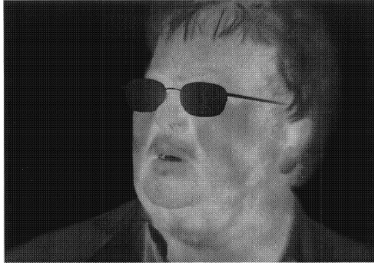
Figure 2.4: Image taken with 1024×768 InSb FPA produced by BAE Systems in collaboration with Defence and Technology Laboratory and Qinetiq Ltd. The field of view of camera and integration time is f/4.5 and 3ms, respectively. Operating temperature of the FPA is 77 K [67].
