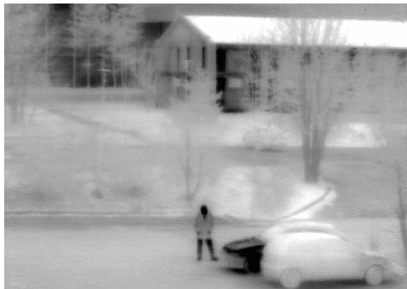
Figure 7.10: Outdoor thermal image taken with the InP/InGaAs QWIP FPA at 70 K sensor temperature.
