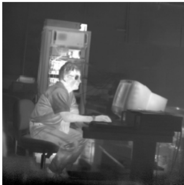
Figure 2.5: Image obtained from megapixel MWIR HgCdTe FPA of LETI [41].
