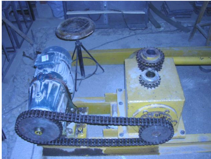
Figure 3.3 Electric motor, gearbox system, eccentric disks and the rigid shaft
