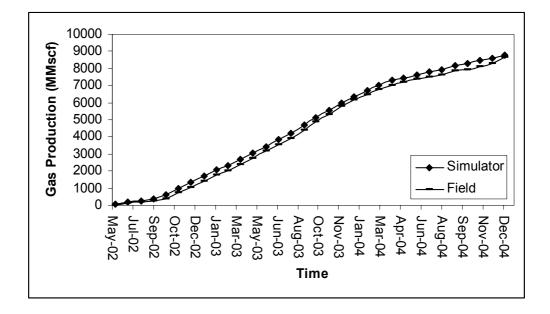
Figure 6. 23. Comparison of Total Gas Production of the field at the end of Simulation
