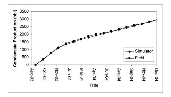
Figure 6. 12. Comparison of Condensate Production for W2
