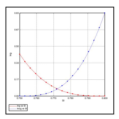
Figure 4. 2. Gas Relative Permeability and Oil relative permeability to gas versus total liquid saturation
