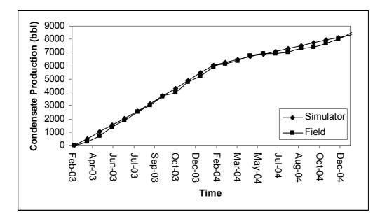
Figure 6. 14. Comparison of Condensate Production for W4
