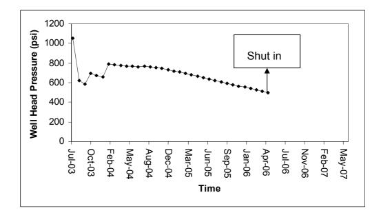
Figure 7. 32. Well Head Behavior of W2 during Scenario 4
