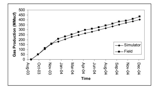
Figure 6. 7. Comparison of Gas Production for W2
