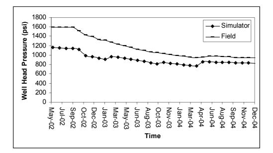
Figure 6.1. Comparison of Well head pressure for W1
