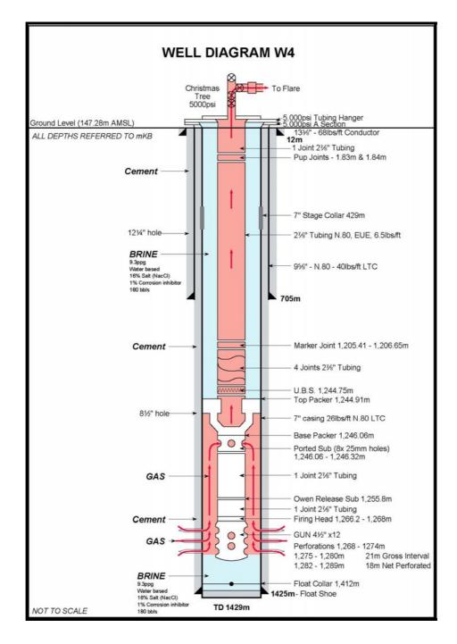
Figure E. 4. Well Diagram of W4
