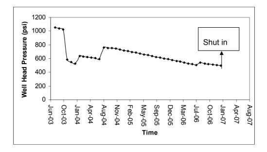
Figure 7. 14. Well Head Pressure Behavior of W2 during Scenario 2
