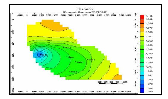
Figure 7. 9. Reservoir Pressure Distribution at the end of Scenario 2
