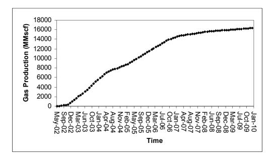
Figure 7. 30. Gas Production during Scenario 4
