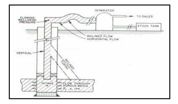
Figure 2.1 Complete Producing System (9)
