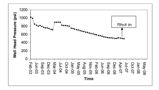
Figure 7. 25. Well Head Pressure Behavior of W4 during Scenario 3
