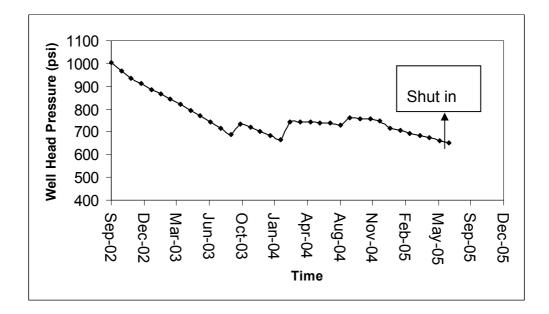
Figure 7. 15. Well Head Pressure Behavior of W3 during Scenario 2
