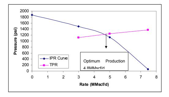
Figure 8. 4. Nodal Analysis applied to W-4
