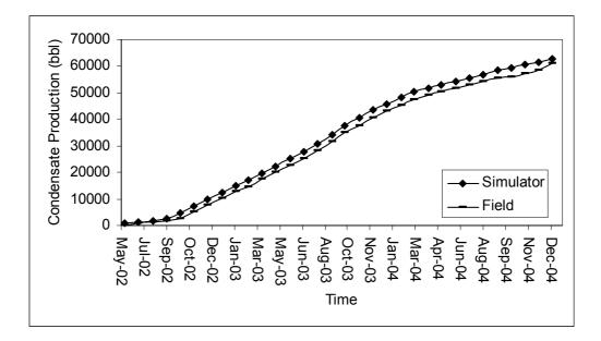
Figure 6. 24. Comparison of Total Condensate Production of the field at the end of simulation.
