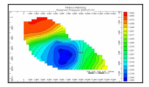
Figure 6. 22. Reservoir Pressure Distribution at the end of Simulation
