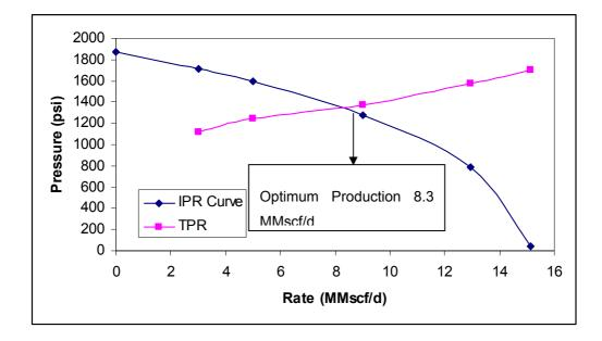
Figure 8. 3. Nodal Analysis applied to W-3
