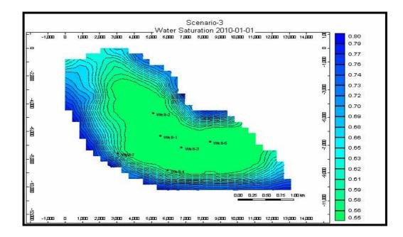
Figure 7. 20. Water Saturation Distribution at the end of Scenario 3
