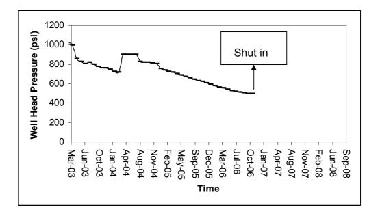
Figure 7. 34. Well Head Behavior of W4 during Scenario 4
