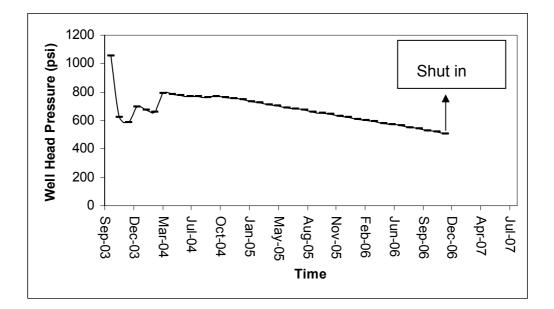
Figure 7.6. Well-head Pressure behavior of W2 during Scenario 1
