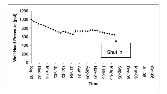
Figure 7 24. Well Head Pressure Behavior of W3 during Scenario 3
