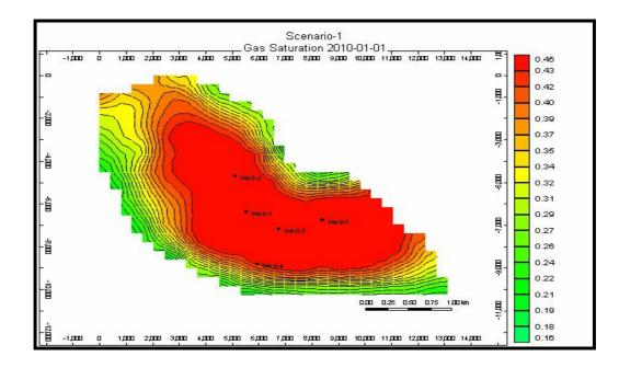
Figure 7.2. Gas Saturation distribution at the end of Scenario 1
