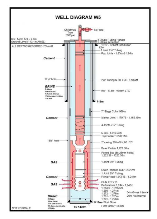
Figure E. 5. Well Diagram of W5
