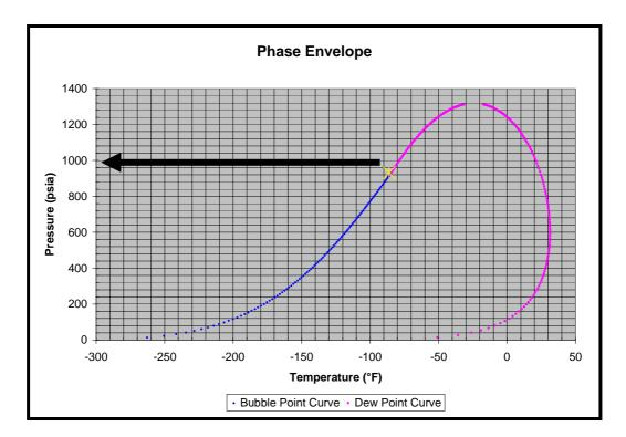
Vleflash Software is used to figure out dew point determination (28)
