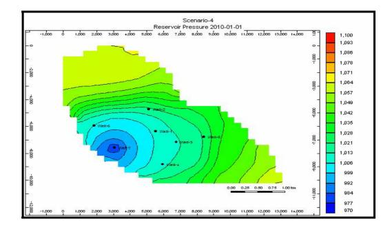
Figure 7. 27. Reservoir Pressure Distribution at the end of Scenario 4
