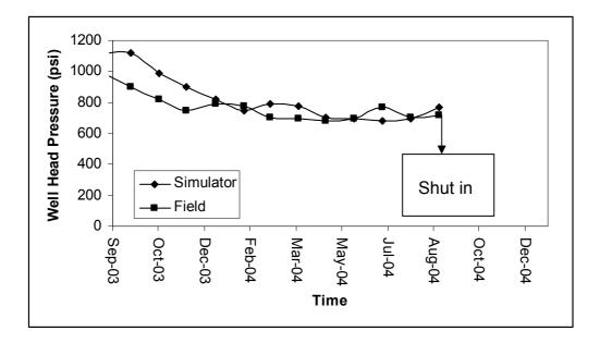
Figure 6. 5. Comparison of Wellhead Pressure for W5
