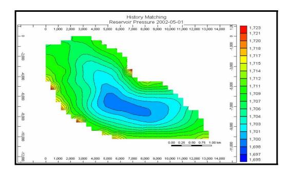
Figure 6. 21. Reservoir Pressure Distribution at Beginning of Simulation
