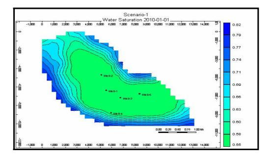
Figure 7. 3. Water Saturation distribution at the end of Scenario 1
