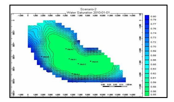
Figure 7. 11. Water Saturation Distribution at the end of Scenario 2
