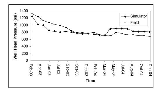
Figure 6. 4 Comparison of Wellhead Pressure for W4
