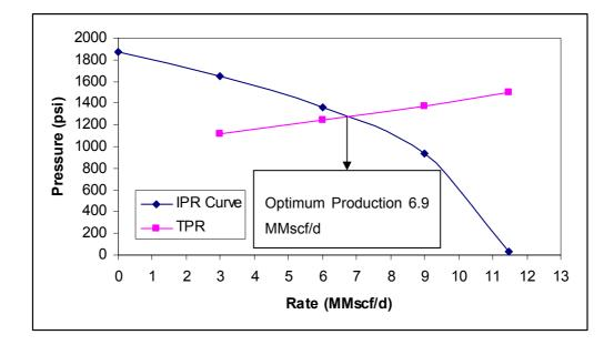
Figure 8. 1. Nodal Analysis applied to W-1
