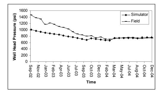
Figure 6. 3. Comparison of Wellhead Pressure for W3
