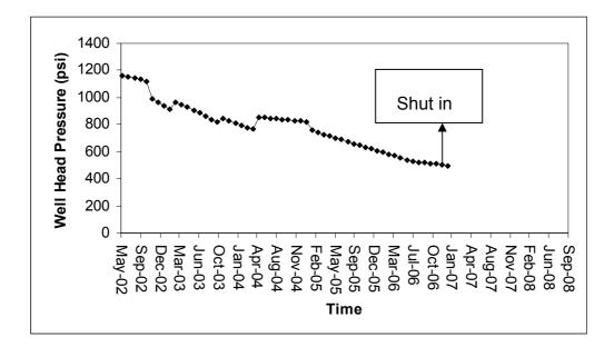
Figure 7. 31. Well Head Behavior of W1 during Scenario 4
