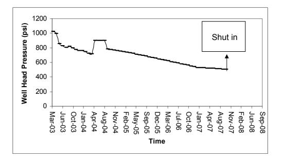
Figure 7. 8. Wellhead Pressure behavior of W4 during Scenario 1
