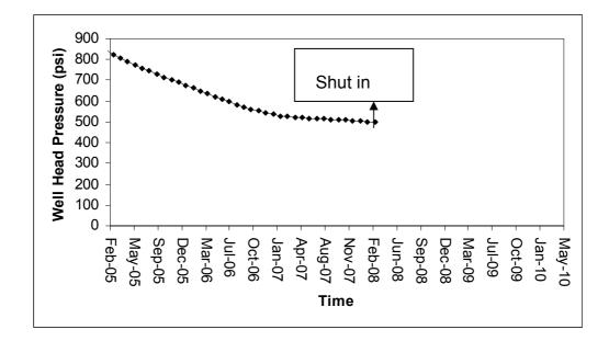
Figure 7. 35. Well Head Behavior of W6 during Scenario 4
