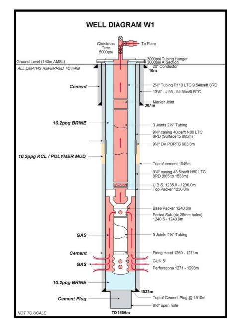
Figure E. 1. Well Diagram of W1
