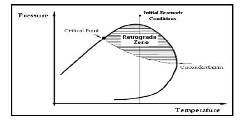
Figure 1.1. Phase Envelope for a typical gas condensate fluid (9)
