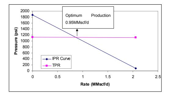
Figure 8. 5. Nodal Analysis applied to W-5
