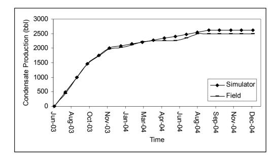
Figure 6. 15. Comparison of Condensate Production for W5
