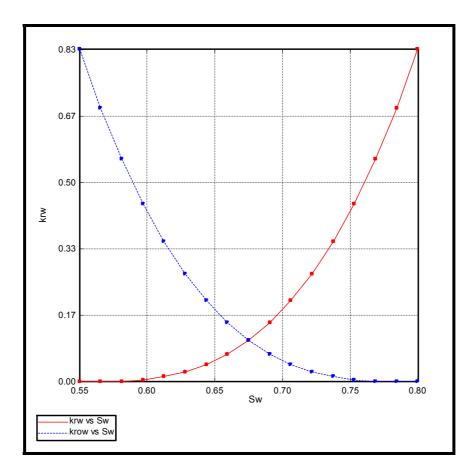
Figure 4. 1. Water Relative Permeability and Oil relative permeability to water versus water saturation
