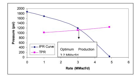
Figure 8. 2. Nodal Analysis applied to W-2
