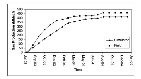
Figure 6. 10. Comparison of Gas Production for W5
