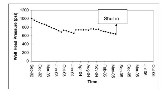
Figure 7. 33. Well Head Behavior of W3 during Scenario 4
