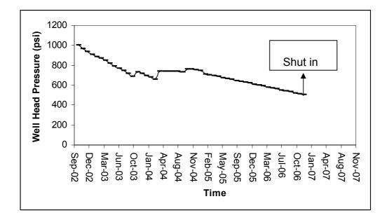
Figure 7. 7. Wellhead Pressure behavior of W3 during Scenario 1
