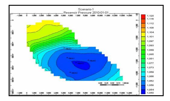
Figure 7. 1. Reservoir Pressure distribution at the end of Scenario 1
