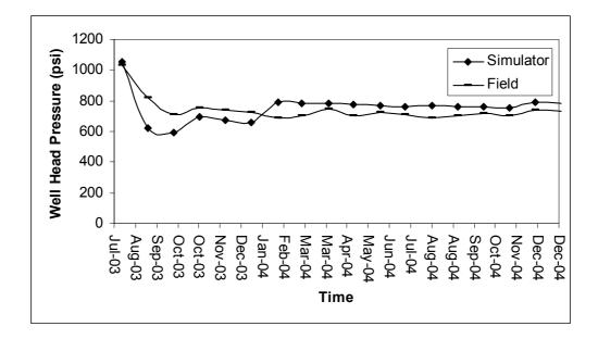
Figure 6. 2. Comparison of Wellhead Pressure for W2
