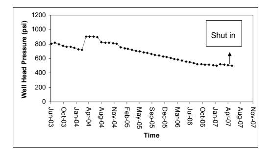
Figure 7. 16. Well Head Pressure Behavior of W4 during Scenario 2
