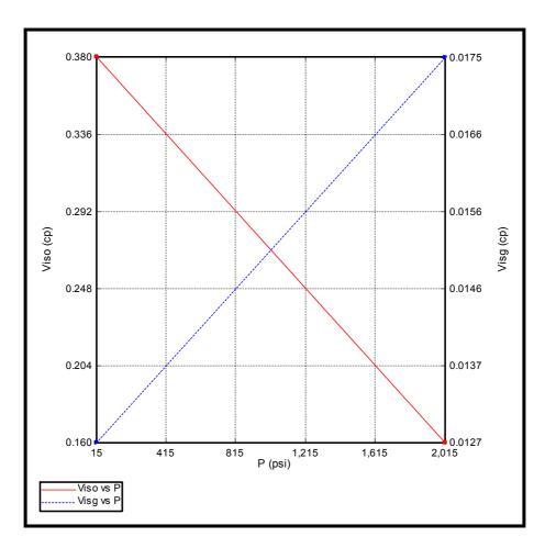
Figure 4. 3. Oil viscosity and Gas viscosity versus Pressure
