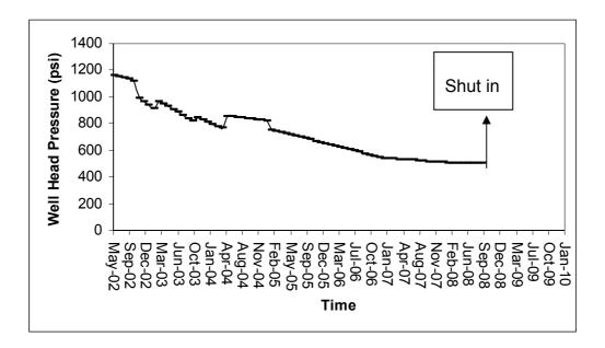
Figure 7. 5. Wellhead Pressure behavior of W1 during Scenario 1
