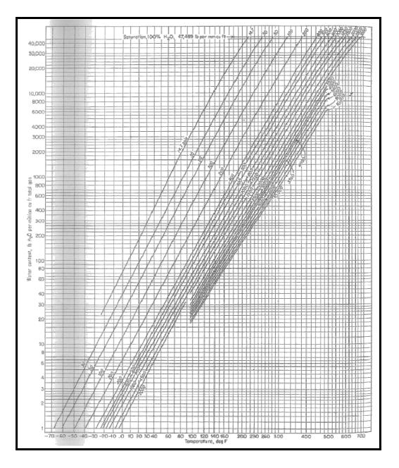
Figure C.6 Water Content of natural gas in equilibrium with water
