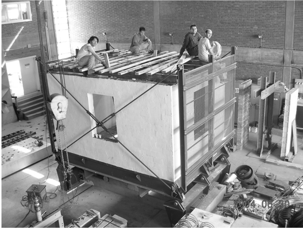
Figure 3.68 Masonry house roof construction
