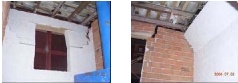
Figure 3.76 Diagonal Cracks on out-of-plane walls (Model #1)
