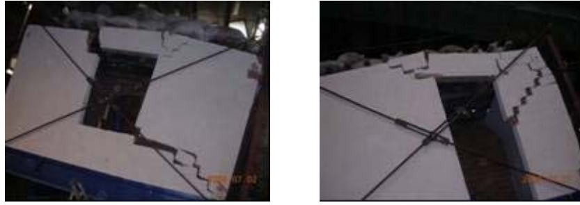
Figure 3.75 Diagonal Cracks on in-plane walls (Model #1)
