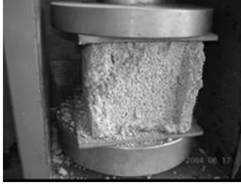
Figure 2.7 Briquette compression test
