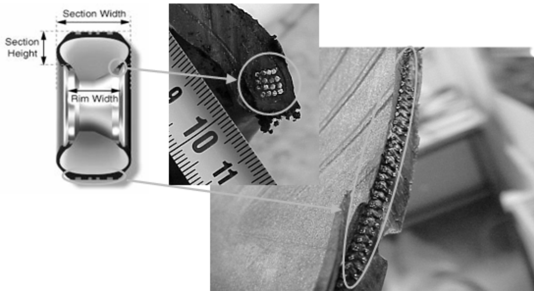
Figure 3.10 Steel wires distribution in rim-rings compared to STR [25]
