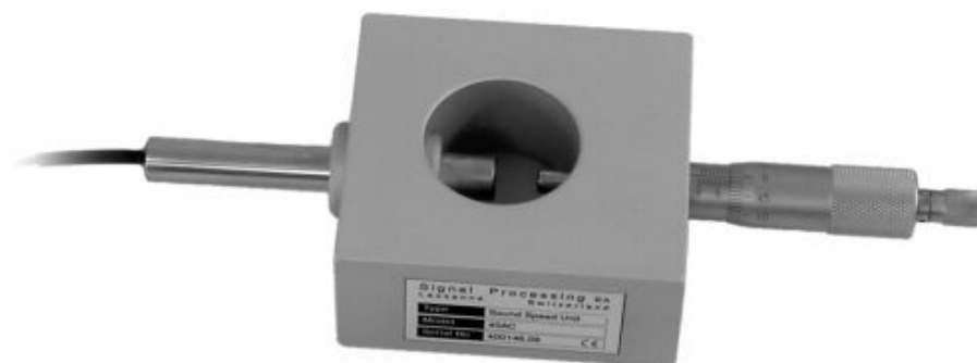
Figure 4.6.1 Sound Speed Measuring Unit
