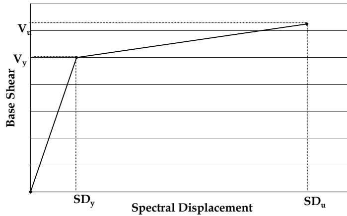
Figure 7.2 - Force - Deformation Relationships for the Building and the Equivalent Single Degree of Freedom System
