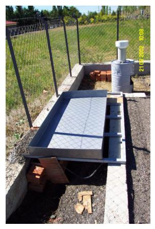
Figure 4.16 Snowmelt lysimeter at Güzelyayla station
