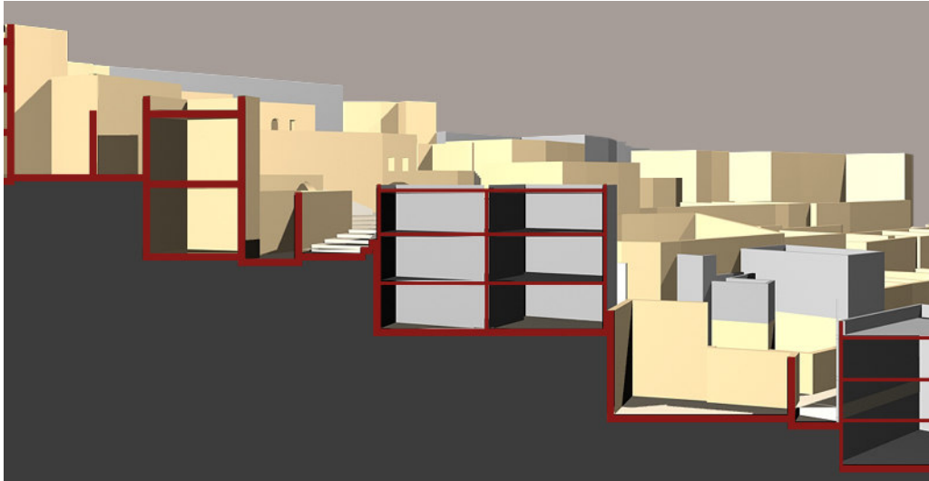
Fig 2.15 Section A3: The incongruent reinforced concrete structure in parcel B. See also view 12 and 22 in Fig 2.12.
