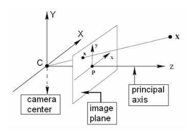
Figure 2.1: Basic pinhole camera geometry
