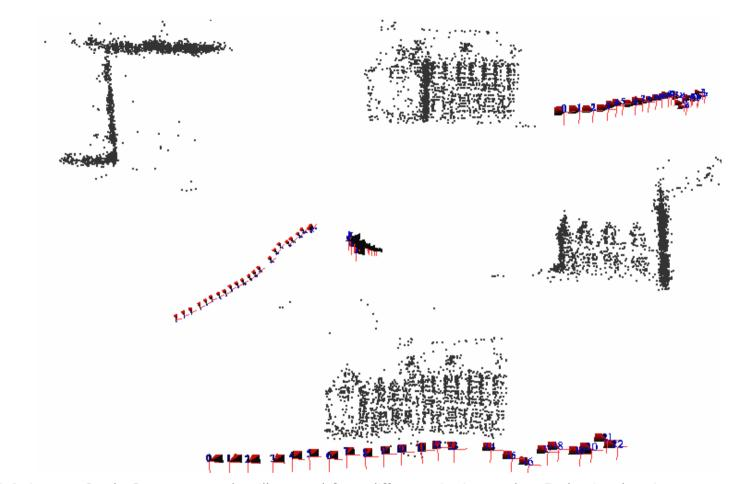
**Figure 4.4:** Leuven Castle Sequence results, illustrated from different viewing angles. Each triangle prism represent a camera location from which a picture is taken.
