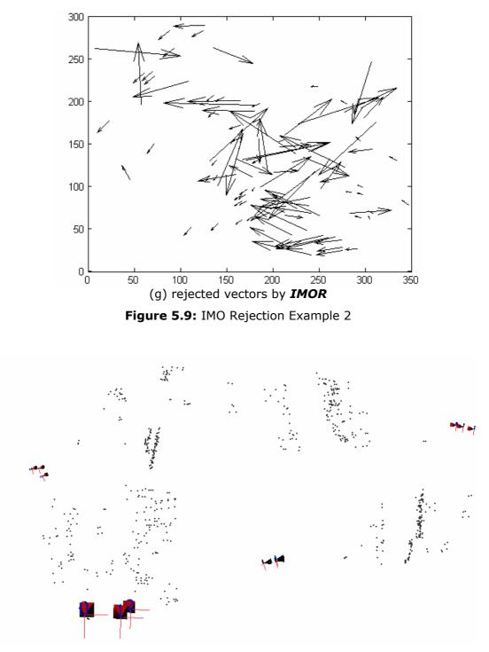
**Figure 5.10:** Reconstruction from images given in Figure 5.9 a, b and c using IMOR+RANSAC algorithm.
