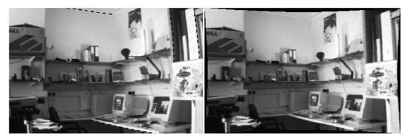
**Figure 2.6:** Radial distortion example [1]: Notice the distortion in the linear lines in the left image. Right image is the corrected one; lines are straight in this image.
