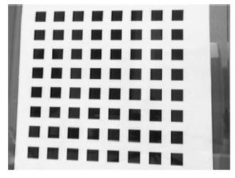
Figure 2.8: 2D Calibration Pattern [6]
