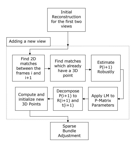
Figure 4.2: Multiple view reconstruction algorithm
