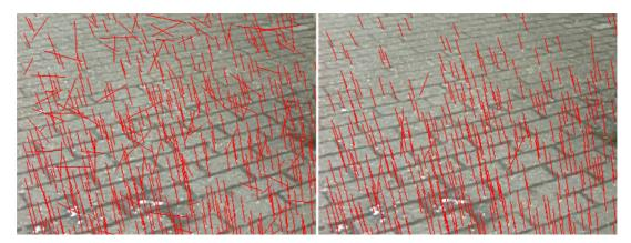
**Figure 3.8:** Comparison of single NCC vs NCC+SM results. In the left image, the results for using only the similarity measure can be observed. In the right image NCC is used together with SM. Most of the outliers due to the repetitive texture of the scene are eliminated.
