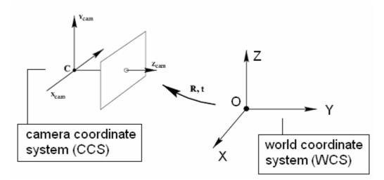
Figure 2.3: Transformation between world and camera coordinate systems
