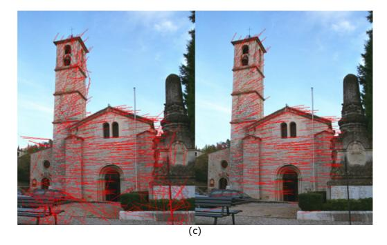
**Figure 3.12:** Examples for RANSAC (a)*BILTEN*, (b) *Lueven Castle*, (c) *Church*: Images on the left show the motion vectors before RANSAC and images on the right show the motion vectors after RANSAC. It can be observed that RANSAC rejects outliers with a good performance.
