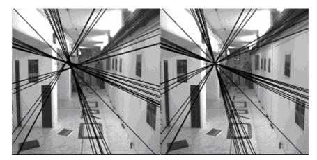
**Figure 3.9:** Rank of the fundamental matrix [1]: Left image shows the epipolar lines for a rank 3 fundamental matrix. Notice that the lines do not converge at a single point. In the right image on the other hand, lines coincide at a single point. Rank-2 constraint has been forced while obtaining this fundamental matrix.
