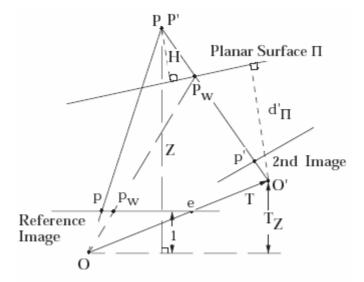
Figure 5.1: Geometric interpretation of the plane+parallax decomposition [60]
