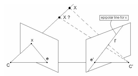
**Figure 2.11:** Back-projected point ambiguity: For a pair of calibrated cameras (*C* and *C*' known), knowing only x will not be sufficient to find the 3D point X.
