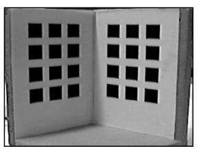
Figure 2.7: A 3D calibration pattern [11]
