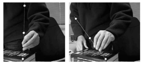
Figure 2.9: 1D calibration pattern [8]
