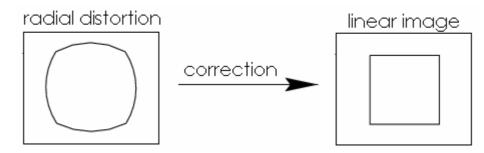
**Figure 2.5** Radial distortion [1]: Left image represents the image before correction and right image is the corrected linear image.
