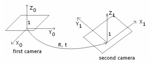
Figure 3.14 : Relative camera positions
