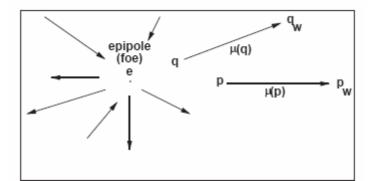
Figure 5.2: Epipolar field of the residual parallax displacements [60]
