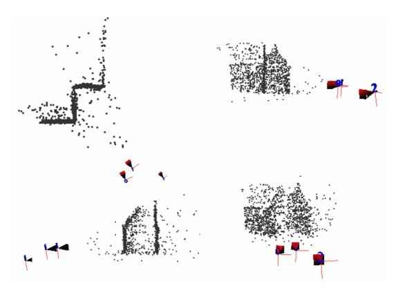
**Figure 5.8:** Reconstruction from images Figure 5.7 (a), (b) and (c) using IMOR+RANSAC
