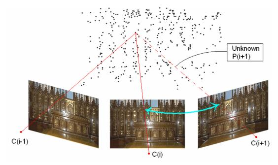
**Figure 4.1:** Pose estimation: 3D-2D correspondences are obtained by using the relation between the structure and the correspondences estimated from frames  $f_i$  and  $f_{i+1}$ .
