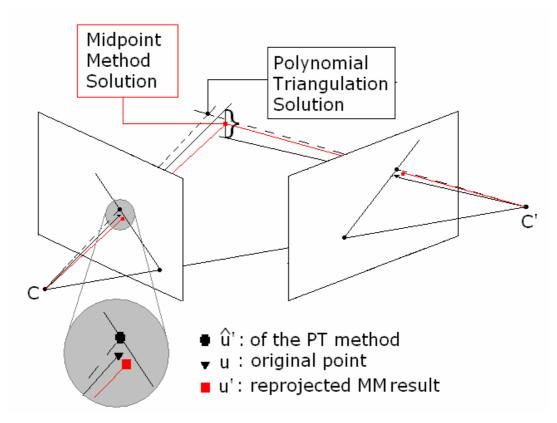
**Figure 3.16:** Polynomial Triangulation (PT): PT finds the closest points on the pencil of epipolar lines and estimates the location of the 3D point using these points. Midpoint method (MM), on the other hand, minimizes the 3D error by selecting the midpoint of the closest point of back-projected rays.
