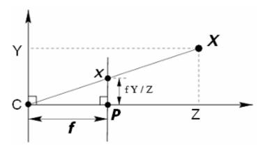
Figure 2.2: Side view of the projection of a 3-D point
