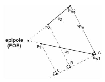
Figure 5.3: Pair-wise parallax-based shape constraint
