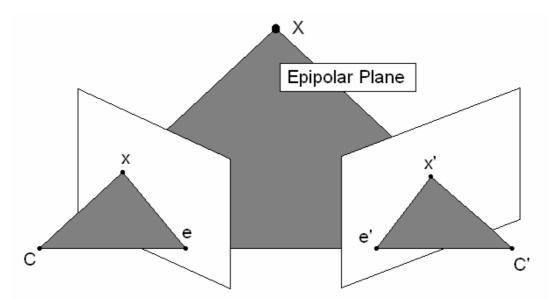
**Figure 2.10**: Epipolar Geometry: *C* and *C'* are camera centers. *X* is any 3D point and x, x' are its projections on different cameras
