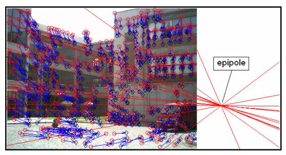
**Figure 3.13:** Displacement vectors between correspondence pairs and the estimated epipole of *BILTEN* image
