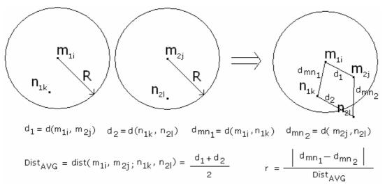
Figure 3.6: Strength measure equations
