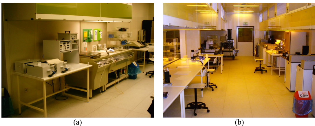
Figure 3.32: (a) Chemical processing hood and (b) lithography area of METU-MET cleanroom, in which the designed gyroscope prototypes are fabricated.
