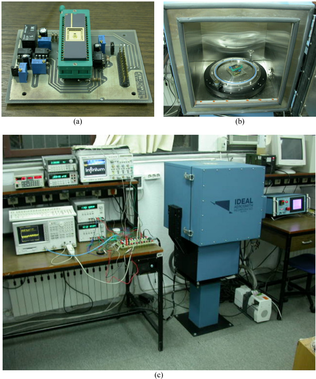
Figure 7.2: The photographs of (a) the gyroscope package mounted on the test PCB, (b) the PCB mounted inside the chamber of the rate table, and (c) the complete test setup showing the measurement equipments used during the tests.
