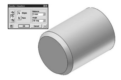
Figure 3.33: Chamfer feature representation.
