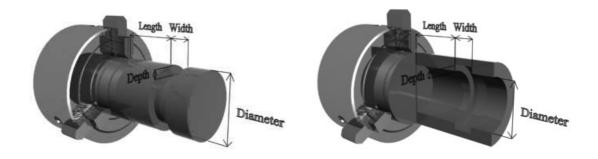
Figure 3.12: Groove feature parameters.
