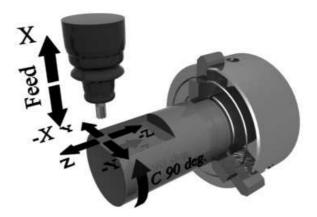
Figure 3.56: NC coordinate system for machining on lateral plane.
