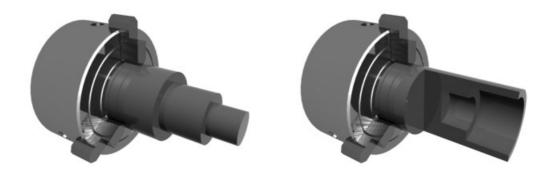
Figure 3.5: Simultaneous cylinder definitions for inner and outer profile.
