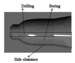
Figure 3.47: Rough inner turning representation.
