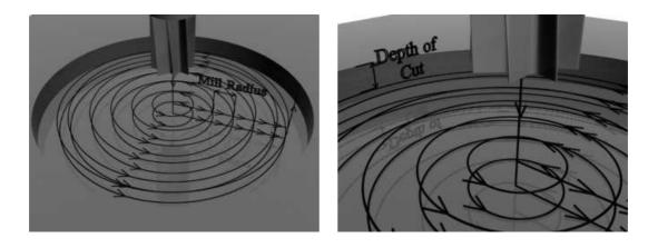
Figure 3.61: Tool path layout for circular pocket milling.
