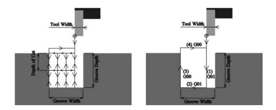
Figure 3.52: Tool path layout for external grooving.
