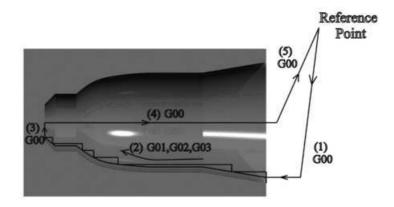
Figure 3.50: Final cut for external roughing.
