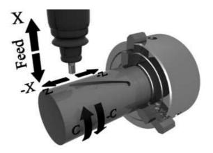
Figure 3.57: NC coordinate system for machining on circumferential plane.
