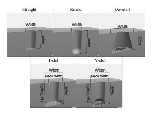
Figure 3.26: Visualization of path cross-sections.
