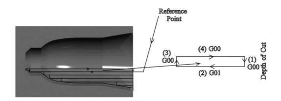
Figure 3.49: Tool path layout for internal roughing.
