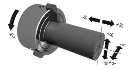
Figure 2.1: Axes of a turning center.
