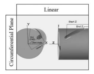
Figure 3.29: Linear path on circumferential plane.
