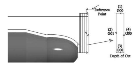
Figure 3.43: Tool path layout for facing.
