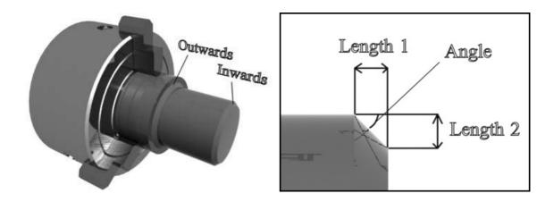
Figure 3.14: Chamfer feature parameters.
