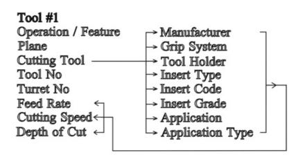
Figure 3.39: Classification of tool definition algorithm.
