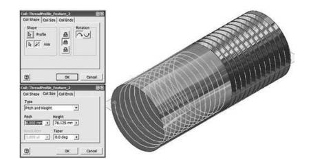
Figure 3.35: Coil feature representation for creating threads.
