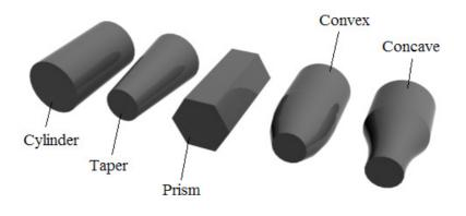
Figure 3.1: Features used to define blank geometry.
