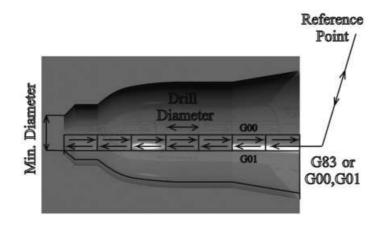
Figure 3.48: Tool path layout for drilling.
