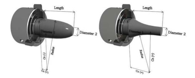
Figure 3.8: Convex and concave feature parameters.
