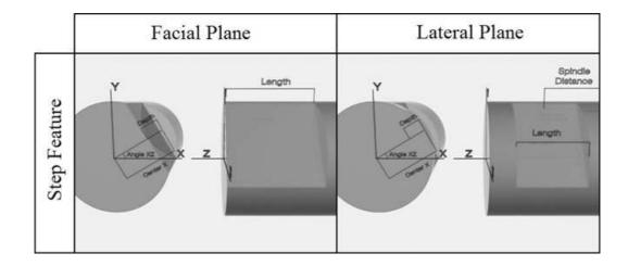
Figure 3.30: Visualization of facial and lateral step feature.
