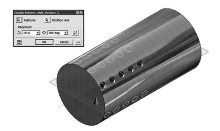
Figure 3.38: Radial patterned hole on circumference plane.
