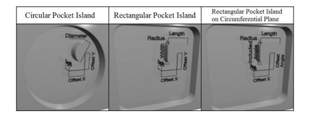
Figure 3.25: Circular and rectangular pocket-island feature on each milling plane.
