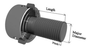
Figure 3.11: Thread feature parameters.
