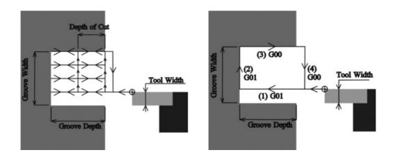
Figure 3.53: Tool path layout for facial grooving.
