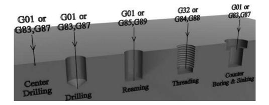
Figure 3.63: Tool path layout for hole milling.
