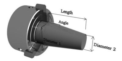
Figure 3.7: Taper feature parameters.
