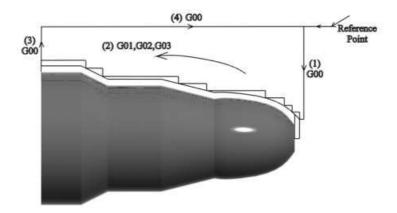
Figure 3.45: Final cut for external roughing.
