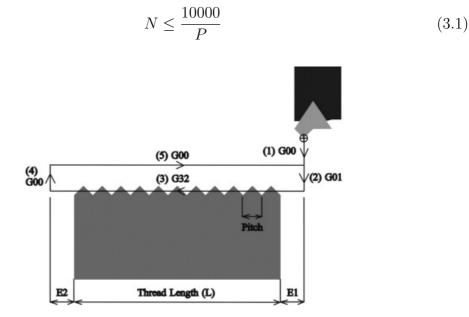
Figure 3.54: Tool path layout for external threading.
