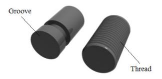
Figure 3.10: Features used to define part turning geometry.
