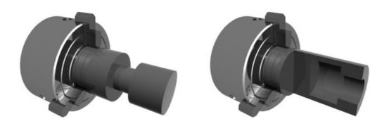
Figure 3.6: Wrong cylinder definitions creating undefined grooves.
