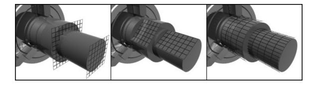
Figure 3.16: Visualization of facial, lateral and circumferential planes.
