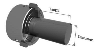
Figure 3.4: Cylinder feature parameters.
