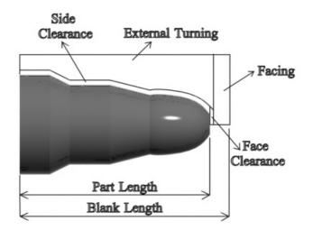
Figure 3.42: Rough outer turning representation.
