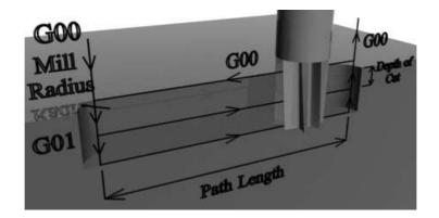
Figure 3.62: Tool path layout for path milling.
