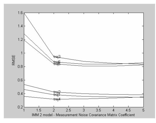
Figure 5.3.4 RMSE vs. 2-model IMM Filter Meas. Noise Cov. Matrix Coef.
