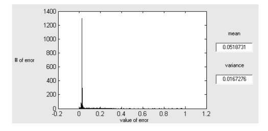
Figure 5.2.4.6 Error Distribution of EKF Output
