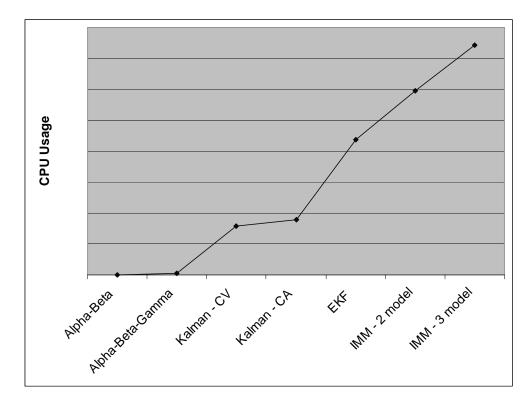
Figure 4.2.2 CPU Usage of Estimation Filters
