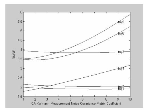
Figure 5.3.2 RMSE vs. CA Kalman Filter Meas. Noise Cov. Matrix Coef.
