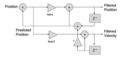
Figure 2.3.1.1 Block diagram of Alpha-Beta Filter
