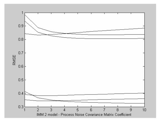
Figure 5.3.8 RMSE vs. 2-model IMM Filter Proc. Noise Cov. Matrix Coef.
