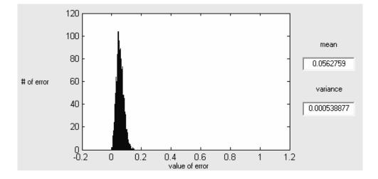
Figure 5.2.1.5 Error Distribution of CA Kalman Filter Output
