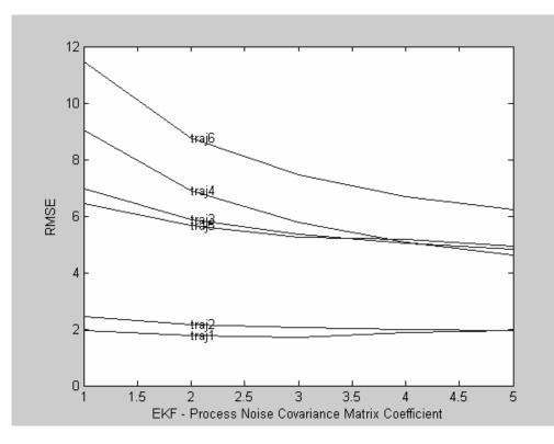
Figure 5.3.7 RMSE vs. EKF Proc. Noise Cov. Matrix Coef.
