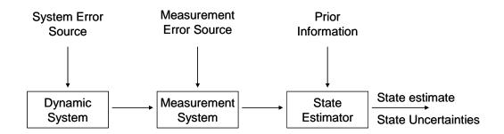
Figure 2.1.2 Block diagram of State Estimation
