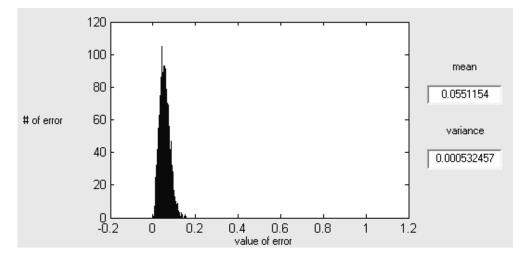
Figure 5.2.4.5 Error Distribution of CA Kalman Filter Output
