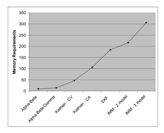
**Figure 4.1.1 Memory Requirements of Fundamental Estimation Filters**
