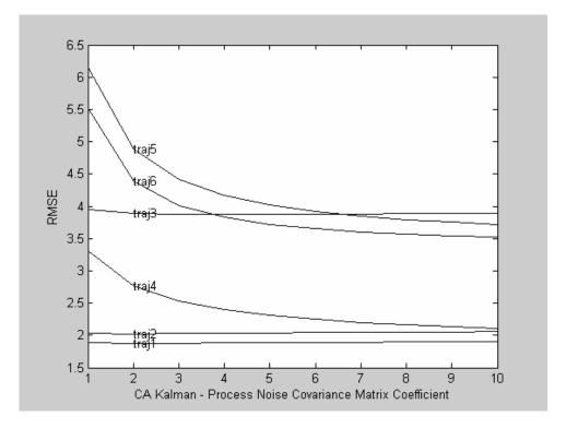
Figure 5.3.6 RMSE vs. CA Kalman Filter Proc. Noise Cov. Matrix Coef.
