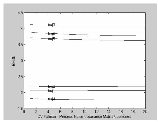
Figure 5.3.5 RMSE vs. CV Kalman Filter Proc. Noise Cov. Matrix Coef.
