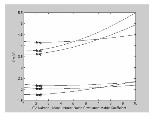
Figure 5.3.1 RMSE vs. CV Kalman Filter Meas. Noise Cov. Matrix Coef.
