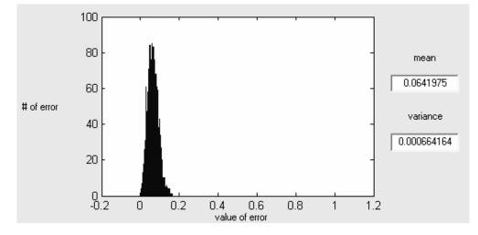
Figure 5.2.6.5 Error Distribution of CA Kalman Filter Output
