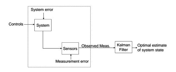
Figure 2.3.1 Typical Kalman Filter Application [9]
