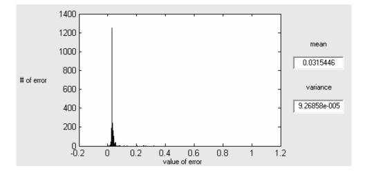
Figure 5.2.1.6 Error Distribution of EKF Output
