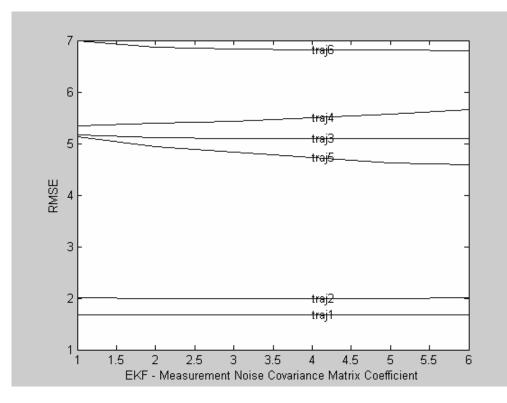
Figure 5.3.3 RMSE vs. EKF Meas. Noise Cov. Matrix Coef.
