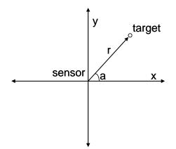
Figure 3.4.1 Sensor Measurement Vector
