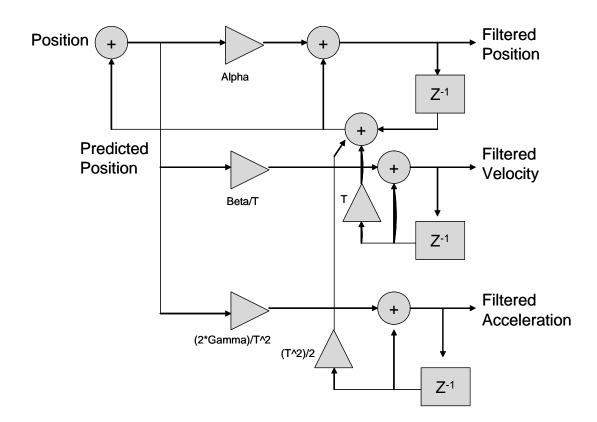
Figure 2.3.2.1 Block diagram of Alpha-Beta-Gamma Filter
