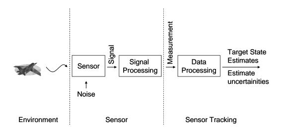
Figure 2.2.1 Block diagram of typical Tracking System
