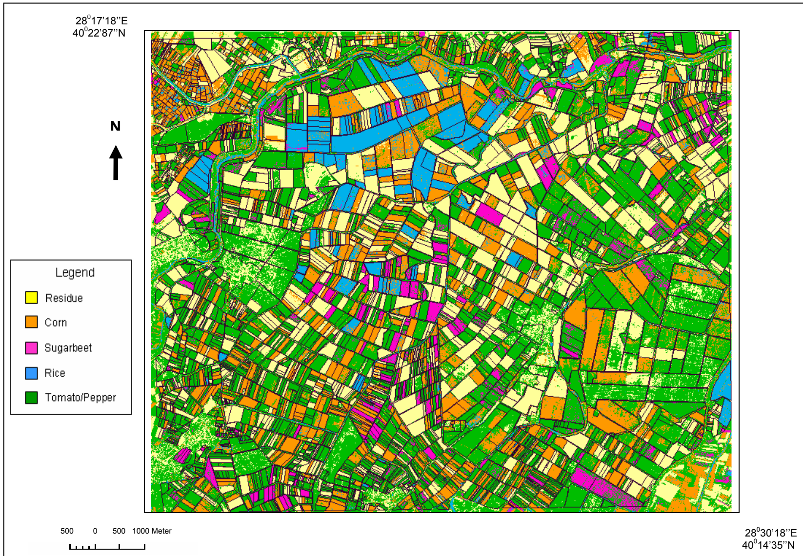
Figure G.3 The output of the post-polygon classification for the IKONOS XS image using common bands
