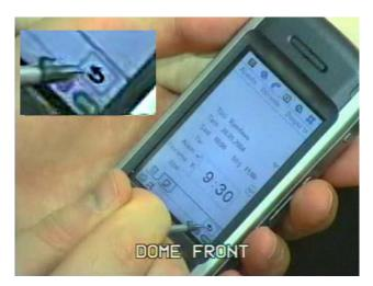
Figure 4.12 The return button for saving a calendar entry (Thumbnail image edited for visual clarity)
