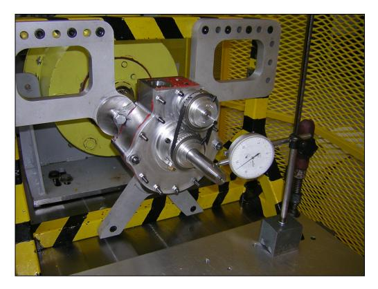
Figure 3-7 Photograph of the Manufactured Rotary Compressor
