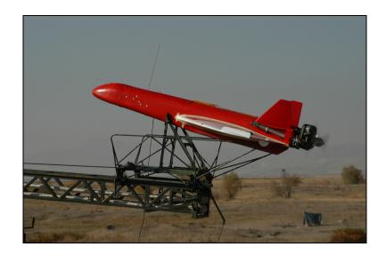
Figure 2-13 Turna, TAI's Unmanned Air Vehicle
