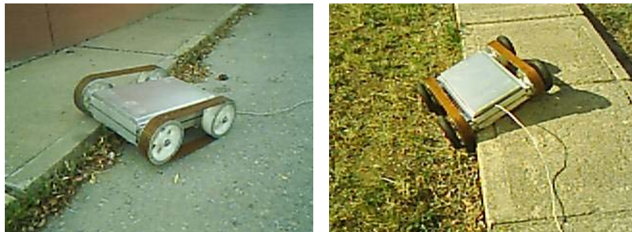
Figure 5.4 Tracked robot base crosses over a step
