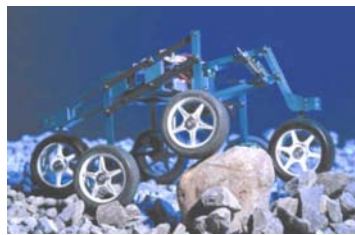
Figure 2.7 Shrimp having six motorized wheels [Lauria, 1991]
