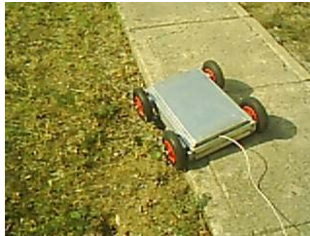
Figure 5.3 Wheeled robot base crosses over a step
