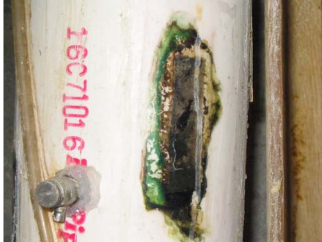
Figure 4.34. Section 35 cm from the top of the filter showing aerobic anaerobic transition (black region indicate anaerobic region) (10 th set in which HLR: 4 m 3 /m 2 .day, COD inf : 150 mg/L, Chl-a inf : 250 µg/L)
