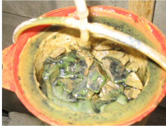
Figure 4.30. Top view from the model trickling filter (6 th set in which HLR: 2 m 3 /m 2 .day, COD inf : 150 mg/L, Chl-a inf : 600 µg/L)
